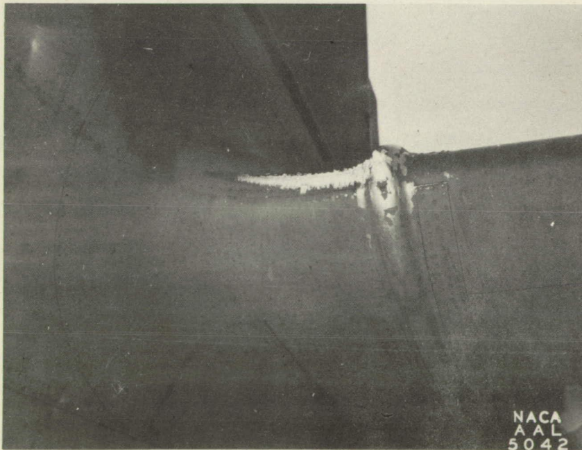
Figure 15.- Ice accumulation on the left stabilizer splice and fairing of the C-46 airplane. Flight 60. Photograph taken after landing.
