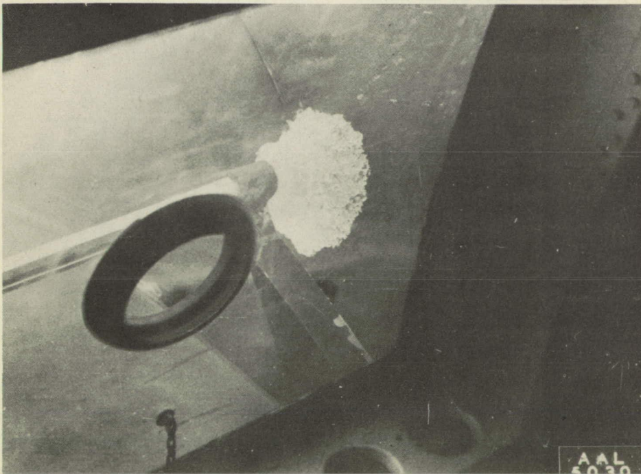
Figure 23.- Ice formation on the left-hand thermometer support, C-46 airplane. Flight 51. Photograph taken in flight.
