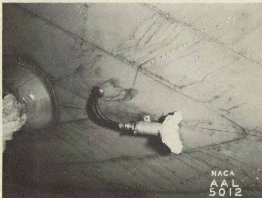
Figure 17. Ice accumulation on pilot's free air thermometer, C-46 airplane. Flight 29. Photograph taken after landing.
