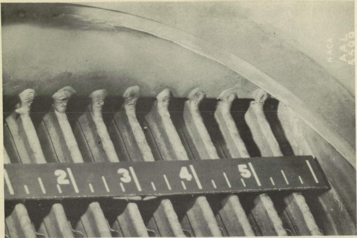
Figure 24.- Left inboard heat exchanger after 100 hours of flight testing. Views showing gas-side cracks and shroud crack, C-46 airplane.
