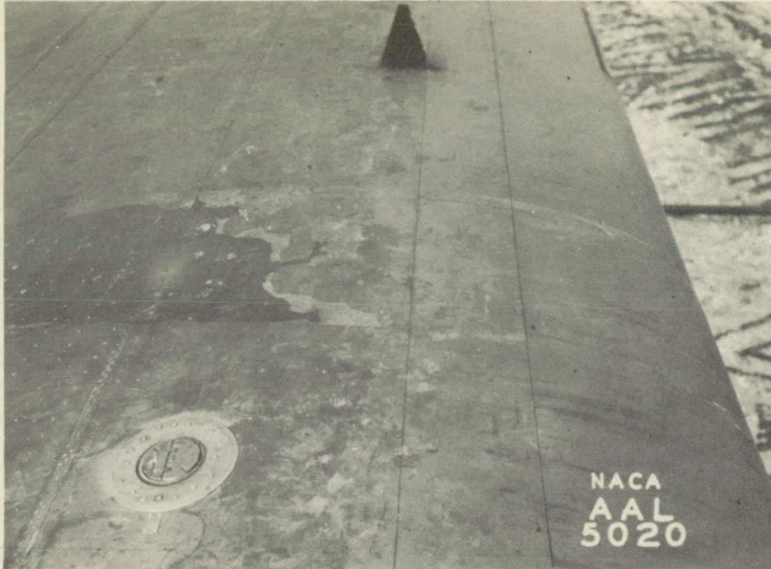
Figure 14.- Ice removed by engine warm-up and take-off in simulated icing tests, C-46 airplane.
