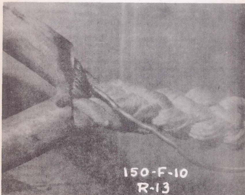
Figure 8.- Damage resulting from arc shown in figure 7. Surface is blackened and some fibers are fused but penetration is very slight.
