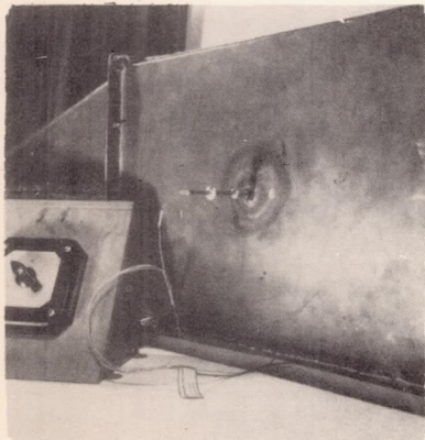
Figure 9.— The traversing thermocouple used to obtain a temperature distribution of the hot air.
