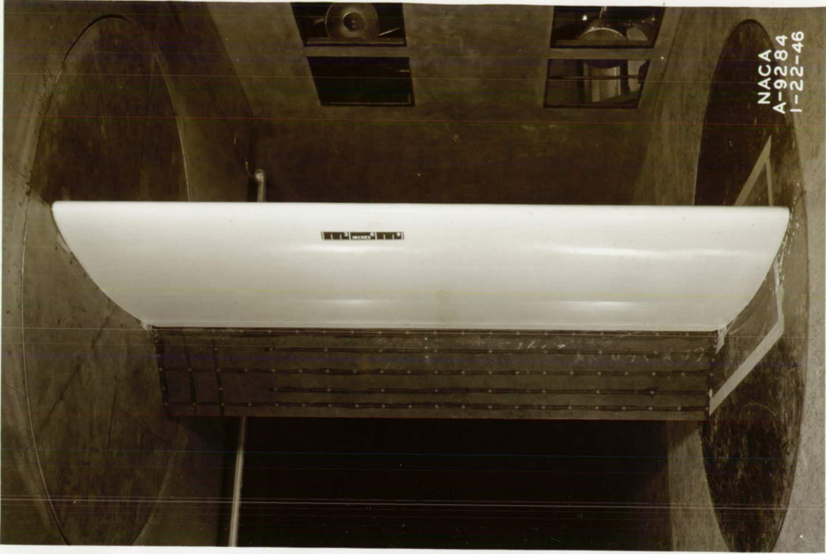
(b) NACA 631-012 airfoil with split flap deflected 40^\circ .
