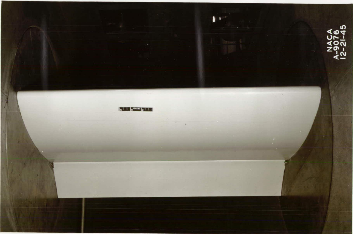
(a) NACA 633-018 airfoil with plain flap deflected 40^\circ .
