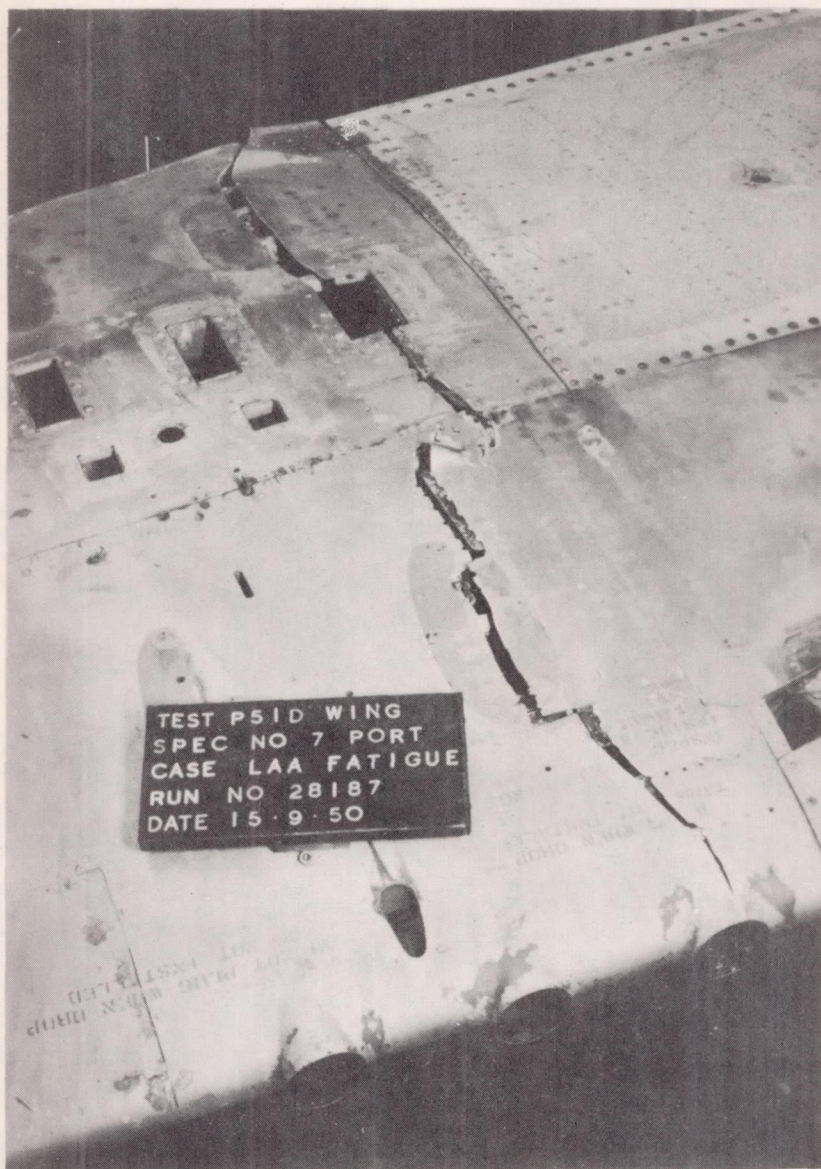
Figure 17.- Failure at station 80 - type I. Outer surface.
