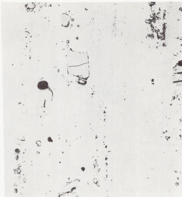
Figure 33.- Alloy "Zicral" of the Aluminum Français (manufacture 1946 or 1947). Angle iron. Large constituents rich in chromium. X160.
