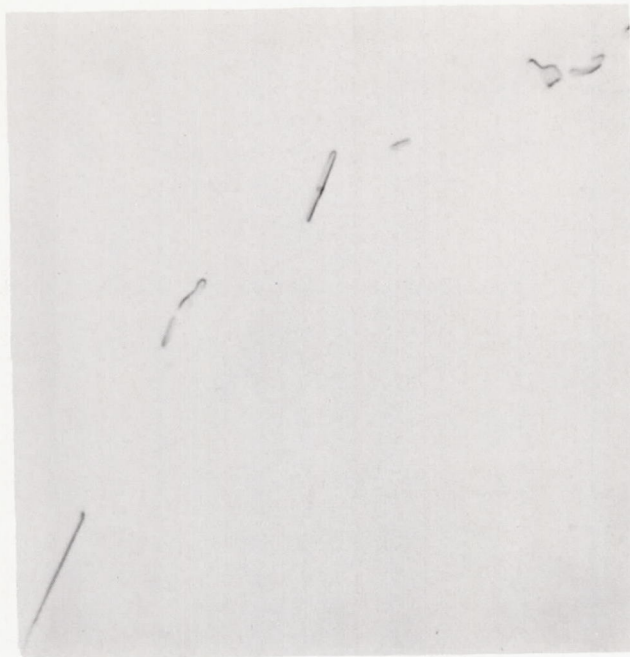
Figure 8.- Constituents in the grain boundaries. X2000.
