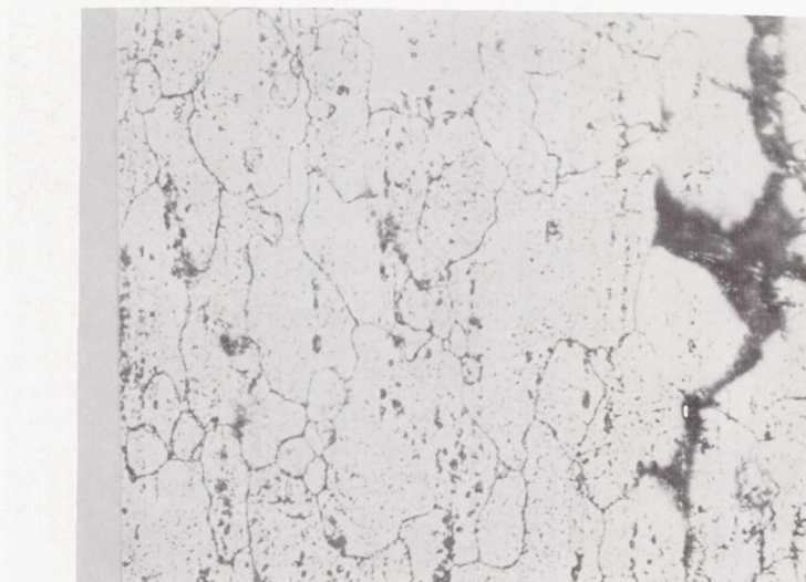
Figure 26.- Exterior surface. Specimen of figure 21. Attack Disa (method no. 2). The anodic oxidation or attack with diluted HF reveal equally the intergranular boundaries. X160.
