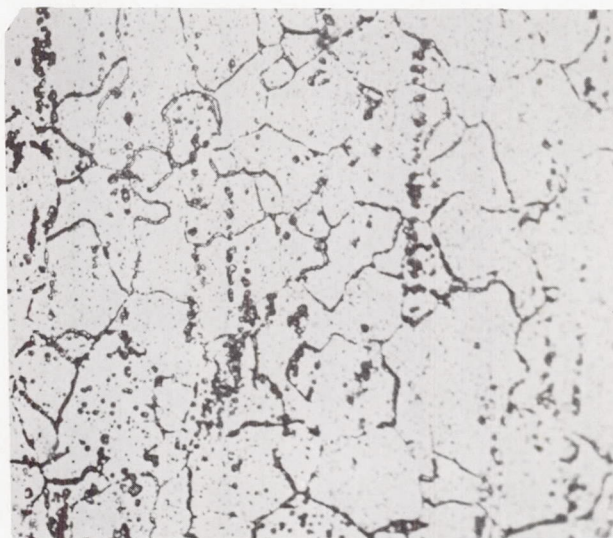
Figure 27.- Exterior surface. Specimen heated at 460°. Attack Disa (method no. 2). Neither anodic oxidation nor attack with diluted HF reveal the intergranular boundaries which are made evident by the Disa attack but appear less continuous than those of the specimen in figure 26. X160.
