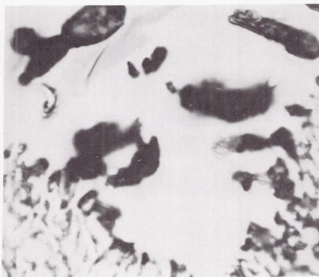
Figure 31.- Specimen of figure 30. Large fragments of silicon and constituents in small plates ( Al_2Cu ?). X2000.
