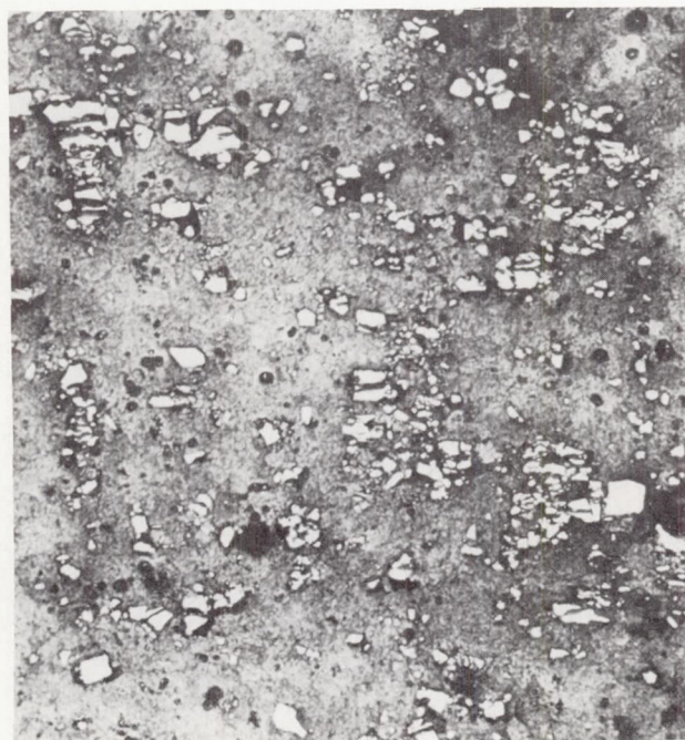
Figure 34.- Alloy T60 of the T.L.H. (manufacture 1944). Sheet metal plate. Polishing followed by attack Disa (method no. 1), leaving non-attacked the large constituents rich in chromium. X160.
