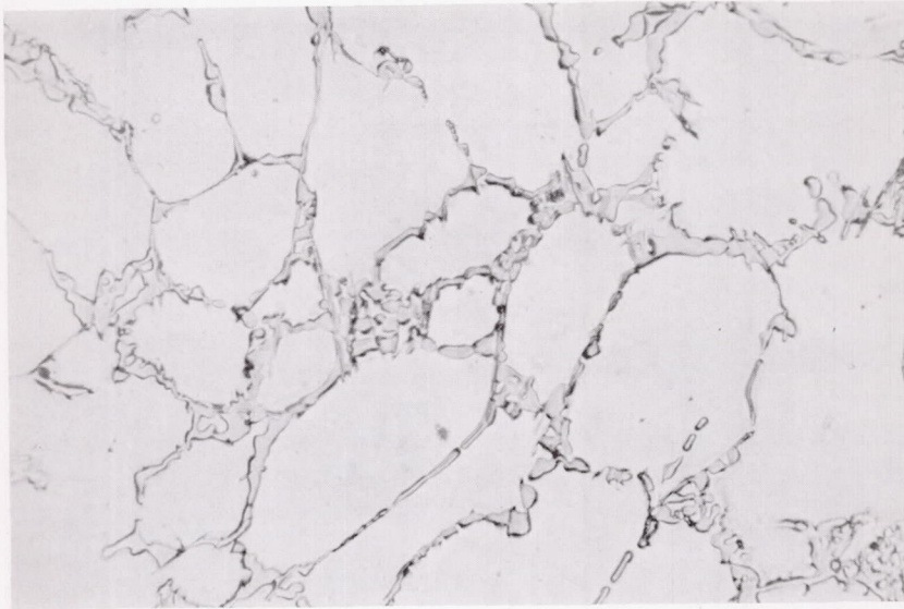
Figure 10.- Alloy Al-Cu (10 percent) chill-cast. Polishing Disa - 45 volts - 20 seconds. X400.
