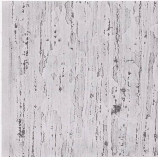
Figure 28.- Section normal to the surfaces of the wall. Specimen of figure 26 - attack Disa (method no. 1). Slight etching of the grains without attack on their boundaries and without pits. X160.
