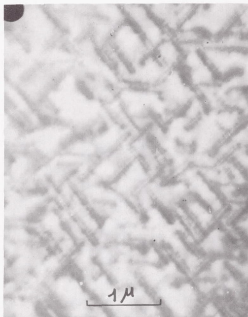
Figure 43.- Alloy Al-Cu 4 percent, tempered 60 hours at 200° C. Direct examination by electron microscope of a section reduced by electrolytical polishing. X20,000.
