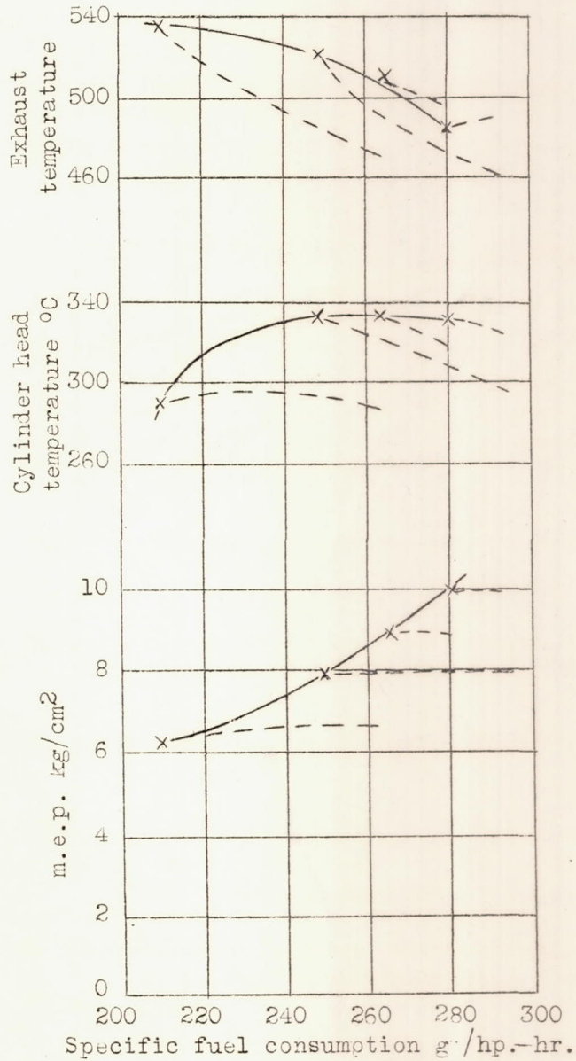
Figure 13.- Airplane engine. Relation between fuel consumption, mean effective pressure, and temperature for different degrees of supercharge.
