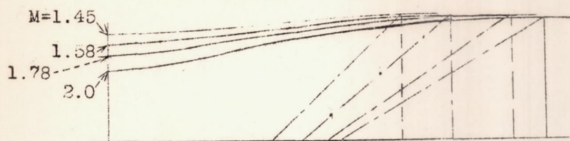
Figure 38.- Nozzle walls for different Mach numbers.
