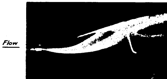
Figure 29.- Rolled up vortex at the side edge of a flat rectangular plate, F/b^2 = 1/1.0 ; \alpha = 18^\circ .
