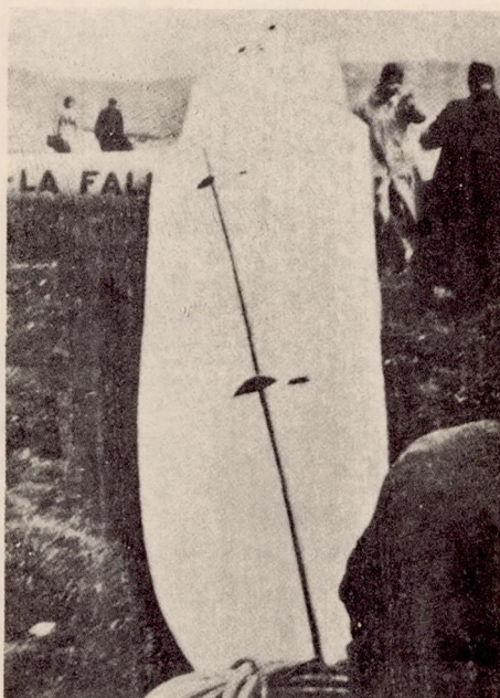
FIG. 14.—Condor, showing aileron chord as large proportion of wing chord at tip
