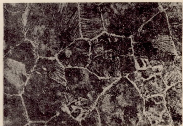
Figure 9a.- Overheat zone of a non-conductive carbon steel; ferrite as net work and Widmannstätten needles.
