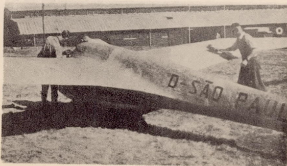
Figure 14.- Wing-fuselage fillet finished (rear view)
