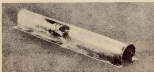
Figure 14.- Arc on control cable housing.
