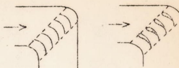
Figures 2a, 2b.-Deflection by guide vanes.
