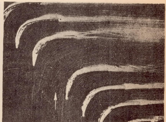
Figure 40.- Flow through gird; one vane removed.
