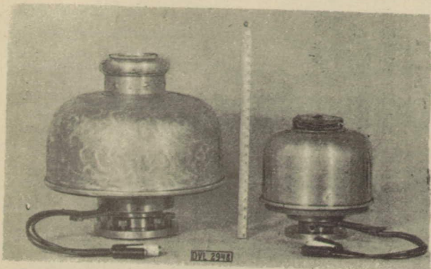
Fig. 4 Small DVL torsionograph, with distance brake, flanged to the crankshaft of an aircraft engine.
