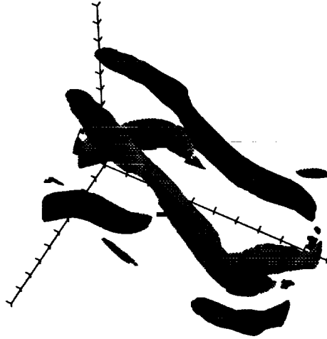
FIGURE 6(c). Three-dimensional structure of streamwise vorticity in Case 3D-2-1 at t = 30 : Surfaces represent 50% of peak value ( \pm 1.9 ), and tic marks are b_{1/2} intervals.
