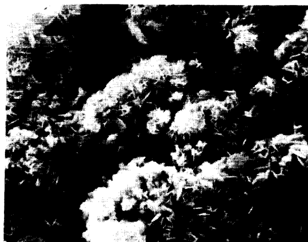
Figure 6. SEM micrograph showing formation of BaCO 3 crystallites on surface of YBa 2 Cu 3 O 7-x specimen stored at 100 percent relative humidity for 2 weeks (magnified 3000 times).
