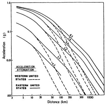
The solid lines are curves used for the eastern region (see text for definition). The dashed lines together with solid lines at close distances are the attenuation curves used for the western region and are taken from Schnabel and Seed (1973).
