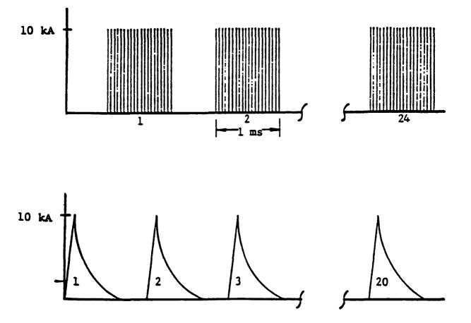
Figure 9.11 A current test waveform composed of 24 bursts (top figure) that are randomly spaced within a 2-s period. Each burst (bottom figure) consists of 20 pulses randomly spaced within a 1-ms period (ref. 9.5).
