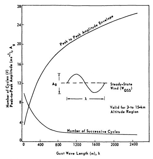
Figure 2-23. Best estimate of expected (≥99 percentile) gust amplitude and number of cycles as a function of gust wavelength.
