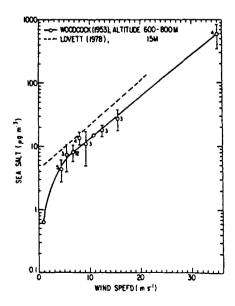
Figure 10.2. Sea-salt concentration at two altitudes as a function of wind speed near the surface of the sea. The number of observations averaged for each data point is given, as well as standard deviation (ref. 10.13).
