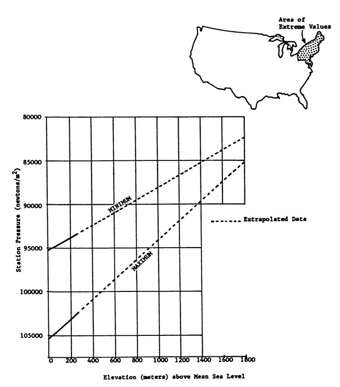
Figure 5.12 Extreme pressure values versus elevation for northeastern United States.
