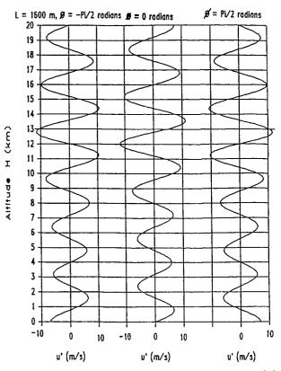
Figure 2-26. Undamped-damped sine gust model.
