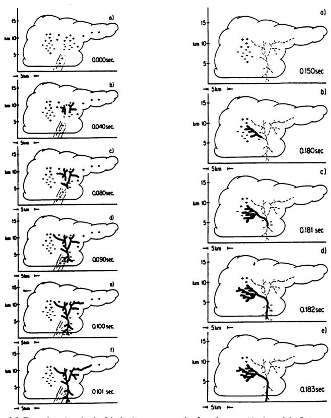
Figure 9.5 First column is a sketch of the luminous processes that form the stepped leader and the first return stroke in a cloud-to-ground lightning flash. Second column shows the development of a lightning dart-leader and a return stroke subsequent to the first in a cloud-to-ground lightning (ref. 9.22).
