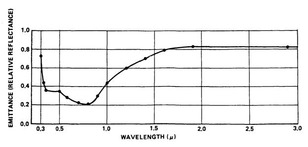
Figure 4.4 Plot of measured emittance of barium sulfate and magnesium oxide (white paint) versus wavelength when exposed to the solar spectrum.
