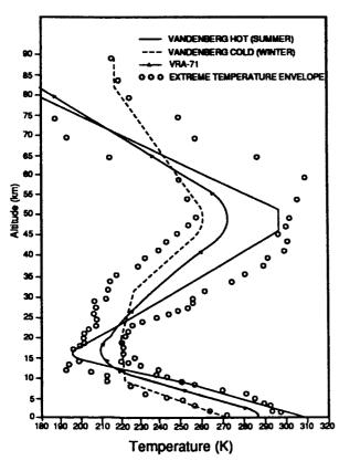
Figure 3.6 Virtual temperture profiles of the VAFB hot, cold, and VRA-71.
