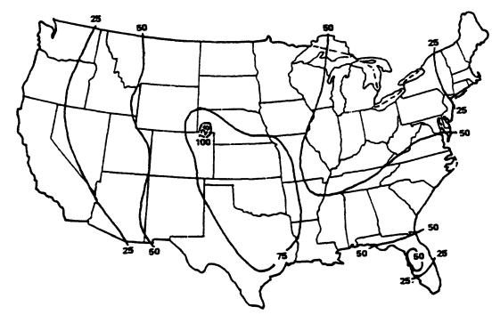
Figure 5.7 Extreme maximum hailstone diameters (mm).
