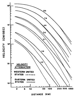
The solid lines are curves used for the eastern region. The dashed lines together with solid lines (in some instances) at close distances are the attenuation curves used for the western region.
