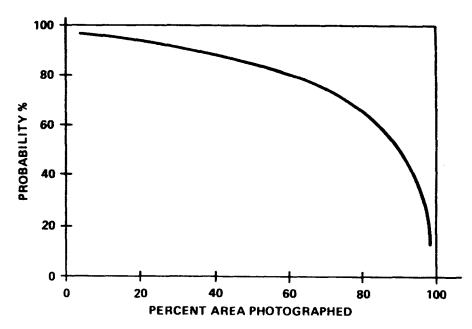
Figure 8.8 Photographic coverage of target area after 10 satellite passes.
