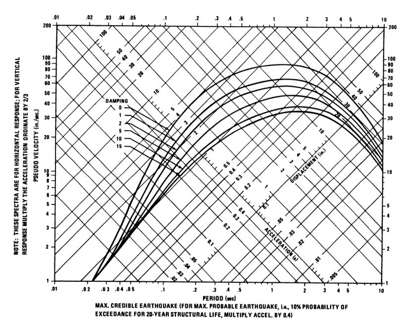
Figure 13.17 0.70E elastic design spectra for strongest potential vibratory ground motion.
