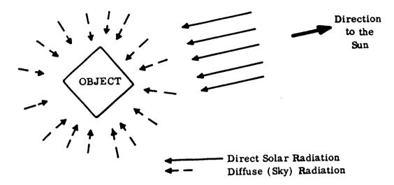
Figure 4.2 Method of applying radiation for design.
