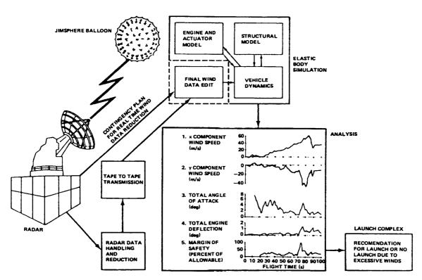
Figure 2-46. Operation of the FPS-16 radar/jimsphere system.
