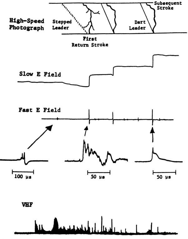
Figure 9.6 Simultaneous photographic and electric field measurements for a multiple stroke, cloud-to-ground lightning flash. The schematic at the bottom is an example of a VHF lightning radiation signature (adapted from ref. 9.10).
