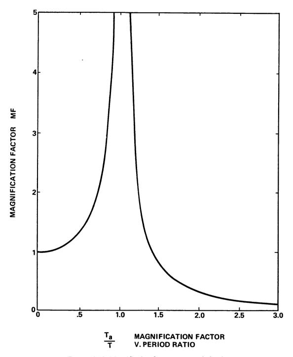
Figure 13.19 Magnification factor versus period ratio.
