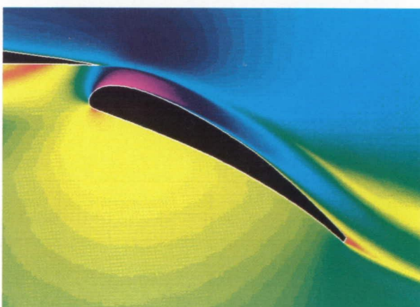
Unstructured grid and Mach number contours for a transport airfoil. Higher than free stream is indicated by the color pink.
