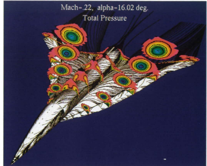
Total pressure contours from the CFL3D solution on the AST-210 configuration.
