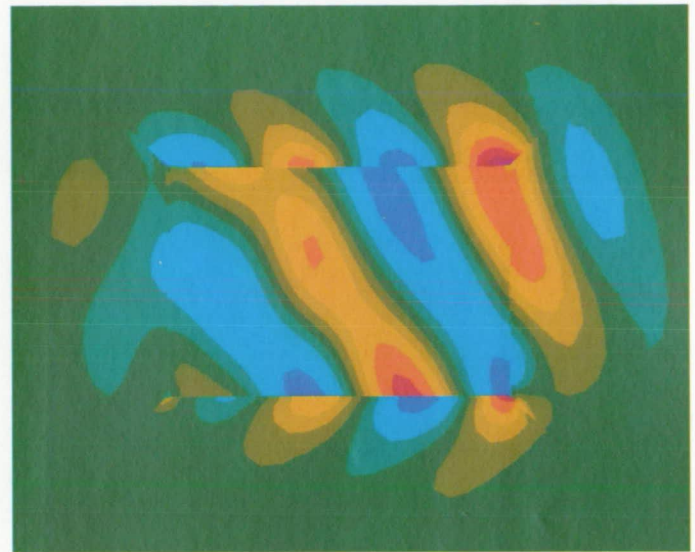
Scattered electric field of a square-aperture inlet for 30 degrees angle of incidence.
