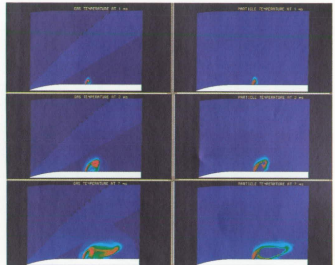
Gas-phase and particle-cloud temperature contours at several times during jet injection.
