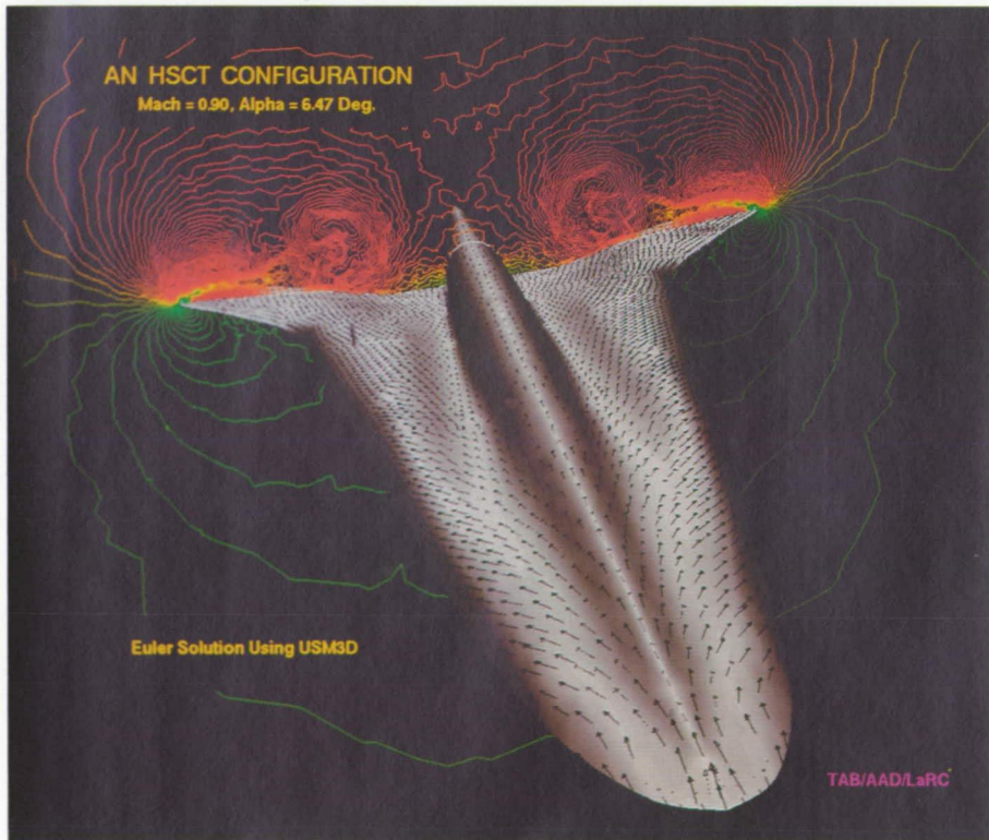
Unstructured-grid solution for a generic High-Speed Civil Transport configuration; M_\infty = 0.901 , \alpha = 6.47 degrees.
