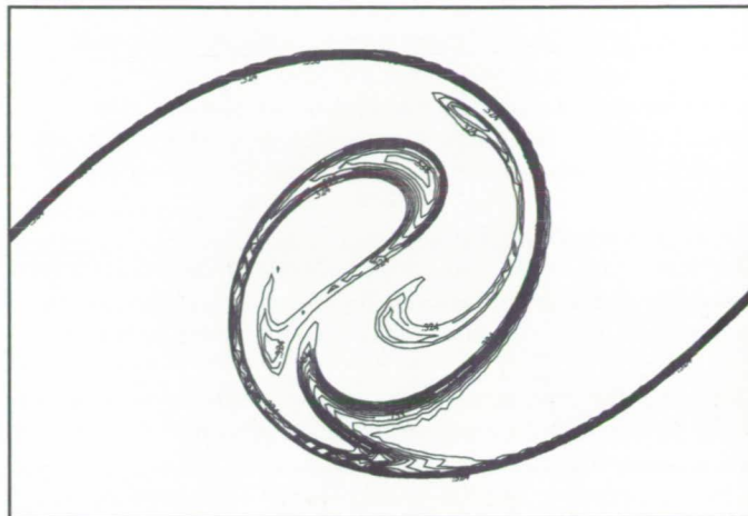
Contours of reactant concentration at the first pairing for two-dimensional simulation with cold reaction; Sc = 0.5 . The highest contour level is 0.92, the lowest is 0.27, and the interval is 0.054.
