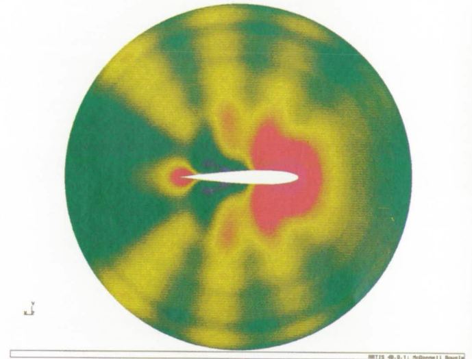
Amplitude of magnetic induction ( B_z ) of a scattered field for the trailing-edge case about the airfoil NACA0012. Red represents maximum amplitude and blue represents minimum amplitude.
