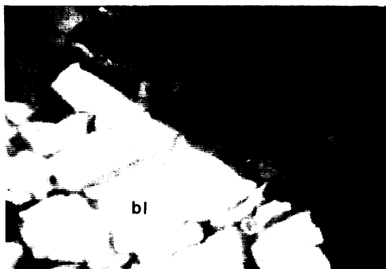
Fig. 1: A black and white photograph of a colar CL image. The light area labeled bl is blue CL enstatite and the dark gray area labeled rd is the red CL enstatite. The dark lines in the light (bl) area are the fractures with red CL. The width of the photograph is 250 micrometers.
