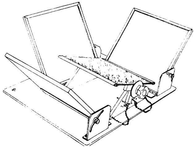
Figure 28. Platform for measuring motor activity of pups.
