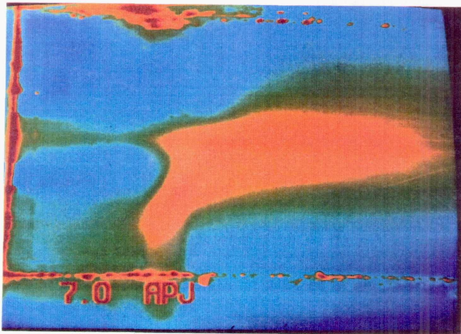
Figure 4.3.1-4. Annular and primary jets with smoke in primary jet, 127 frame average picture, z=7.0 in.
