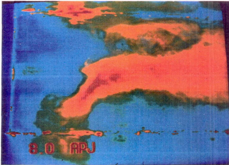
Figure 4.3.1-5. Annular and primary jets with smoke in primary jet, single frame picture, z=8.0 in.
