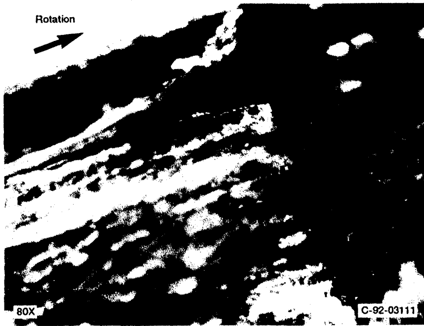
Figure 11.—Rotor leading-edge debris formation (test 2).
