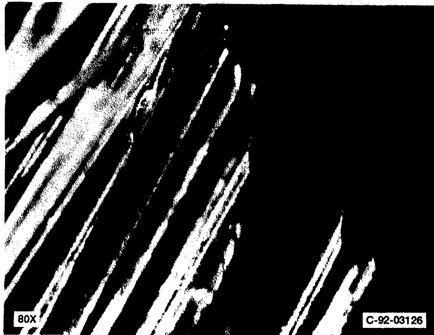
Figure 17.—Brush bristle tips and damage (test 1).
