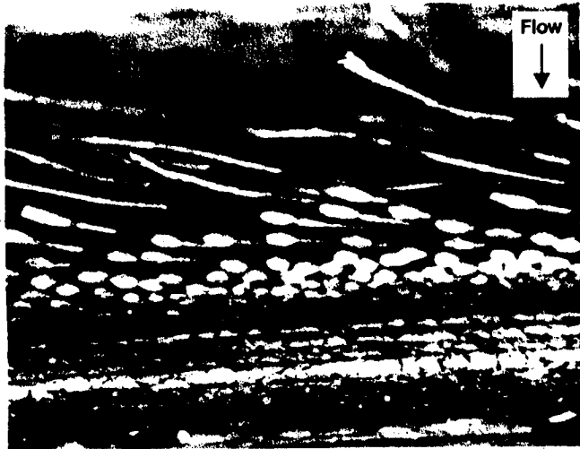
(c) Wear track and fence rub.
