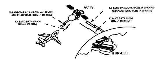
Figure 1 ACTS Broadband Aeronautical Experiment Set-Up
