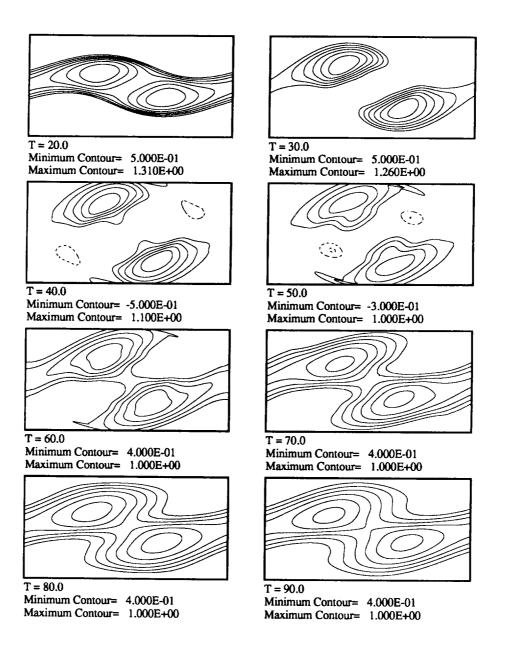
FIGURE 2. (B11 -B22) contours for FENE-P model. Re=50, E=0.5, and b=5.
