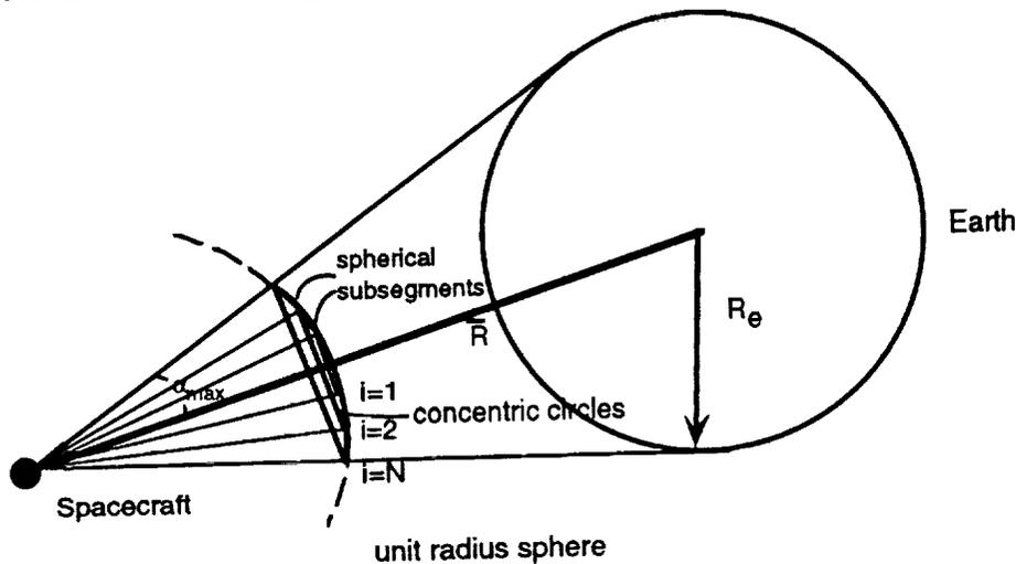
To divide the field of view into  $NA$  equal parts, a set of  $N$  concentric circles ( $i=1,N$ ) is drawn on the spherical segment, where the largest circle corresponds to the horizon of the Earth. Each circle defines another spherical sub-segment and represents the intersection of a cone with the unit sphere.
