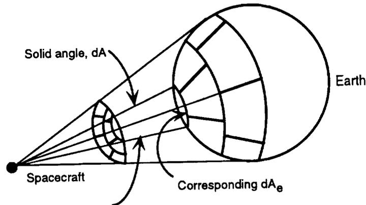
The incremental areas are found by dividing the solid angle subtended by the Earth from the spacecraft's point of view into  $NA$  solid angles of equal size ( $dA$ ), each one corresponding to a piece of the Earth ( $dA_e$ ). Once the areas are defined, the necessary unit vectors are calculated for each area.
