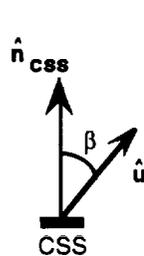
In this case, the incoming light is albedo rather than sunlight, so  $\omega_{CSS} = \omega_{alb}$ , the energy flux due to albedo at the spacecraft's position.
