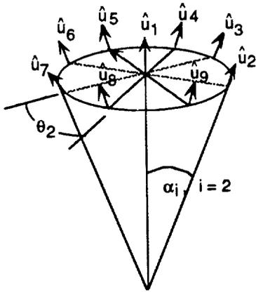
In addition to  $\hat{u}_1$ , define eight more unit vectors at an angle of  $\alpha_2$  from the axis of the field of view cone, equally spaced around the axis in increments of  $\theta_2$ , where  $\theta_2 = \frac{360^\circ}{8}$ .
