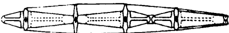
Fig.5d section through the assembly showing the connectors and the bow-string tensioning system
