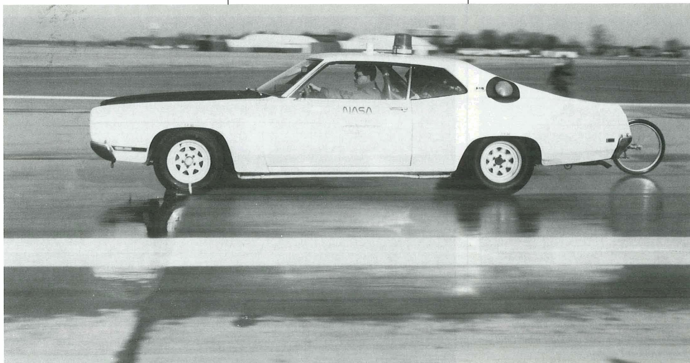
Today, the Ford XL "muscle car" is still part of Langley's runway friction research program.
