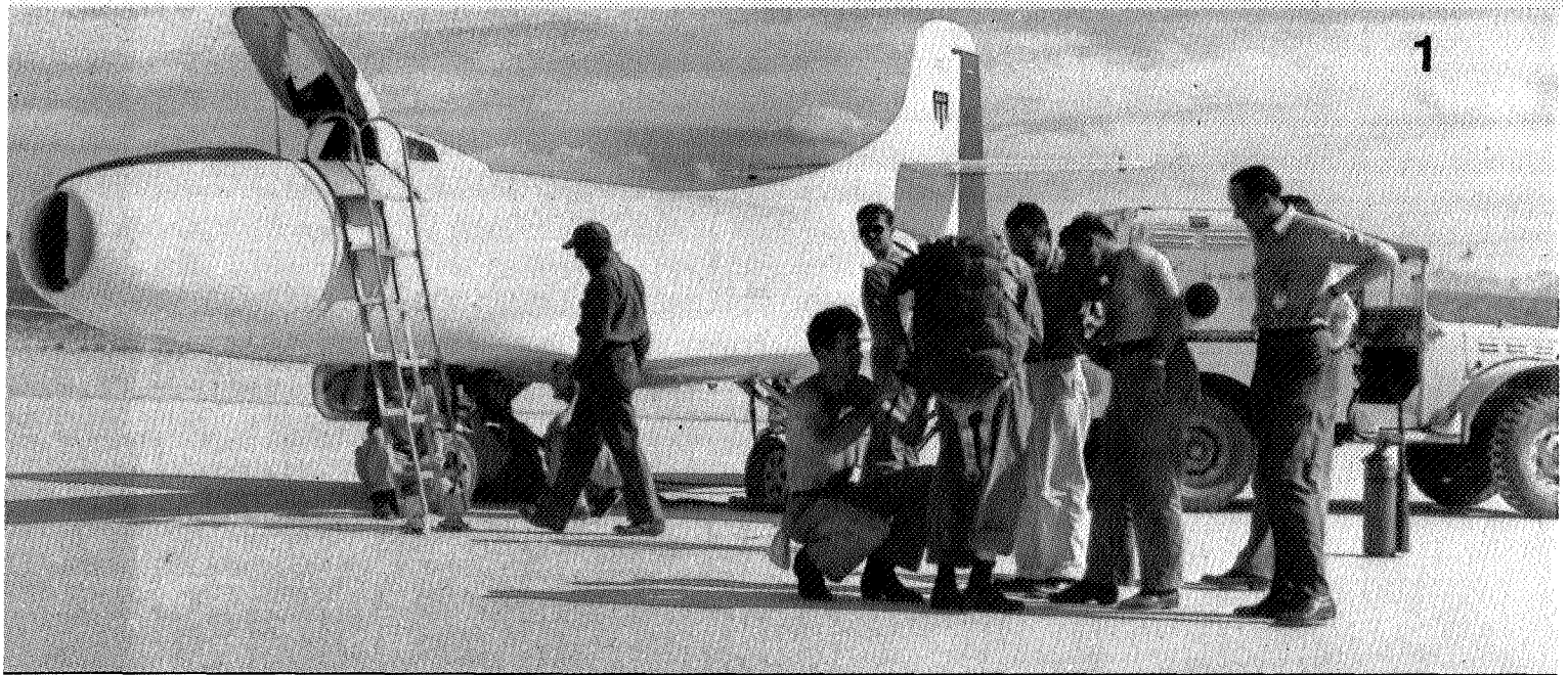
1. The Douglas D-558 Skystreak was another of Champine's mounts. He remembers it as flying well up until Mach .75, with good, stable handling and climb, but as soon as the shock waves hit above Mach .75, it became difficult to control. Designed by Leo Devlin, it had a flight duration of only 30 minutes on its kerosene type fuel, all of it stored in synthetic rubber-lined wing tanks. On May 3, 1948, test pilot Howard Lilly was killed shortly after takeoff, when the Skystreak's engine compressor disintegrated and one of the turbine blades cut through the plane's control cables.
