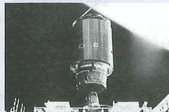
With its perigee kick motor in place, the Intelsat VI satellite spins slowly away from Endeavour's cargo bay.
