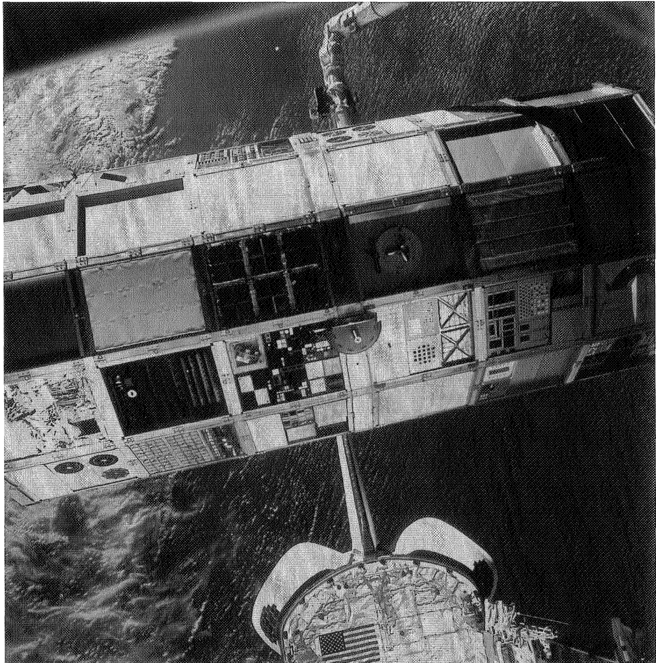
LDEF carried 57 experiments into low-Earth orbit for six years. On board were more than 10,000 items to test the effects of long-term space exposure on spacecraft materials, components, and systems. Pictured is its 1990 retrieval by the Space Shuttle Columbia.
