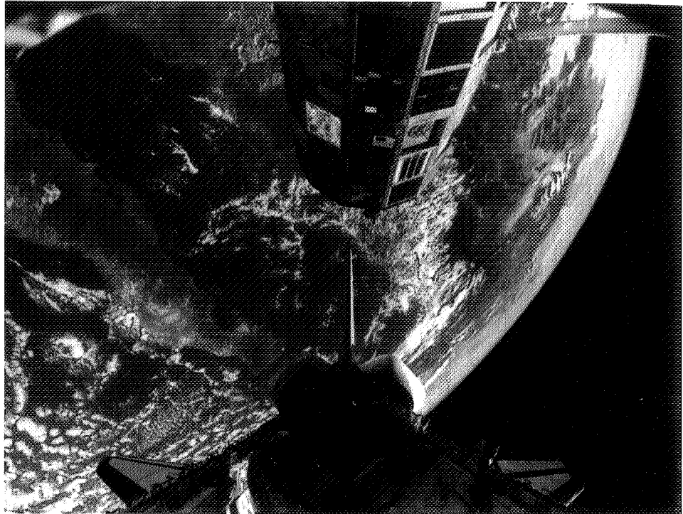
LDEF carried 57 experiments into low-Earth orbit for six years. On board were more than 10,000 items to test the effects of long-term space exposure on spacecraft materials, components and systems. Pictured is its 1990 retrieval by the Space Shuttle Columbia.
