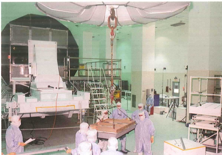
An experiment tray is removed from LDEF in SAEF-2 at the Kennedy Space Center.
