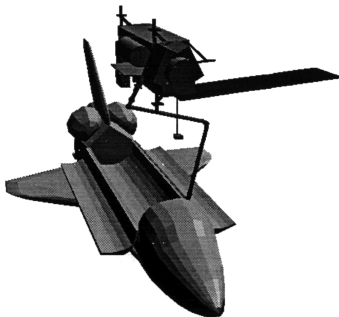
Figure 4.4: The Upper Atmospheric Research Satellite deployed on the RMS in capture/release configuration.
