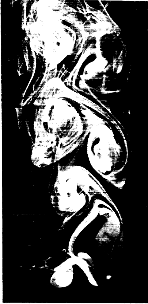
Fig. 1 Hover-jet moving upward into a still air environment (from Ref. 11).
