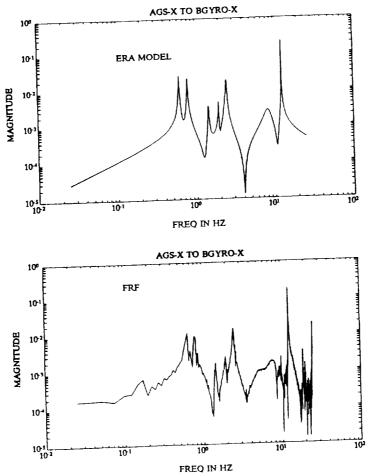
The ERA model for the AGS-X to BGYRO-X loop closely resembles the FRF generated fro test data.
