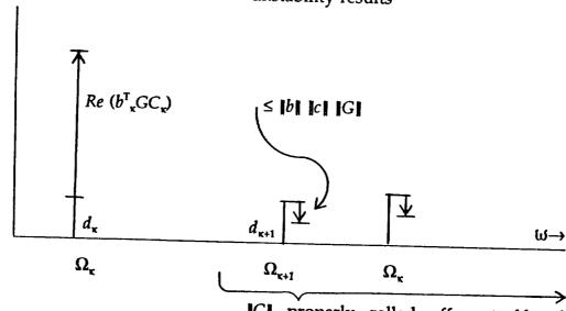
**I**G properly rolled off, out-of-band modes gain stabilized
