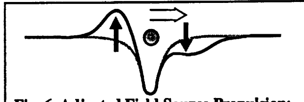
Fig. 6: Adjusted Field Source Propulsion: Similar to differential field propulsion, this version assumes that a symmetric field is initially present and then adjusted asymmetrically to induce a gradient. This version evokes the need to describe fields as having an effective reaction mass.
