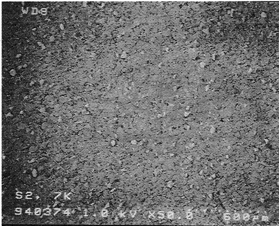
Figure 2. SEM photomicrograph of the lunar ceramic at 50X.
