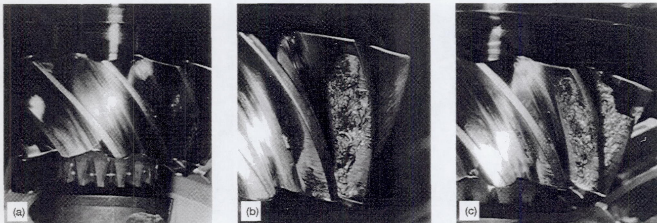
Figure 3.—Pictures of the damaged pinion teeth. (a) 5.5 hr. (b) 12 hr. (c) 17.8 hr.
