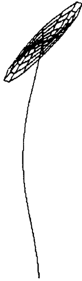
Figure 8.5 Mode shapes 5 and 6: 571.9 Hz.
