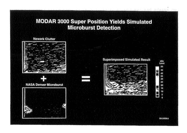
figure 1 <u>Superposition Yields Simulated Microburst Detection in Urban</u>
