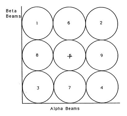
FIGURE 4 3X3 SCAN PATTERN USED FOR AXIAL PASSES
