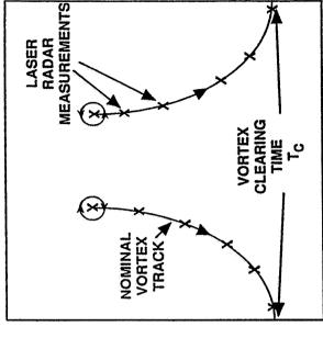
VORTEX DECAY DUE TO TURBULENCE AND WIND SHEAR
