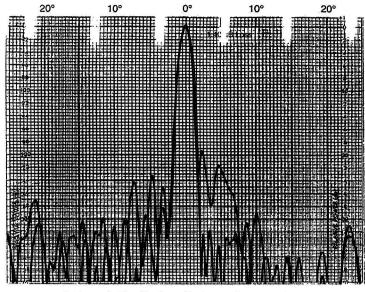
**Azimuth Radiation Pattern Comparison**
