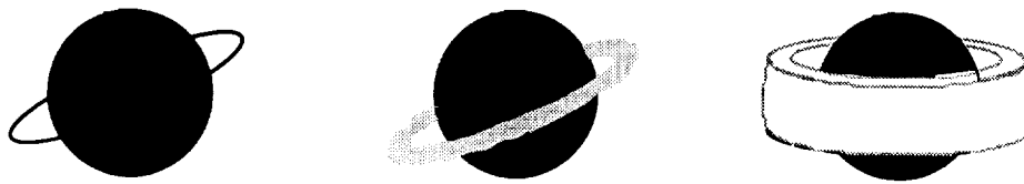
Figure 1: Over time, the cloud of debris that results from a fragmentation event will expand and eventually encompass the Earth.
