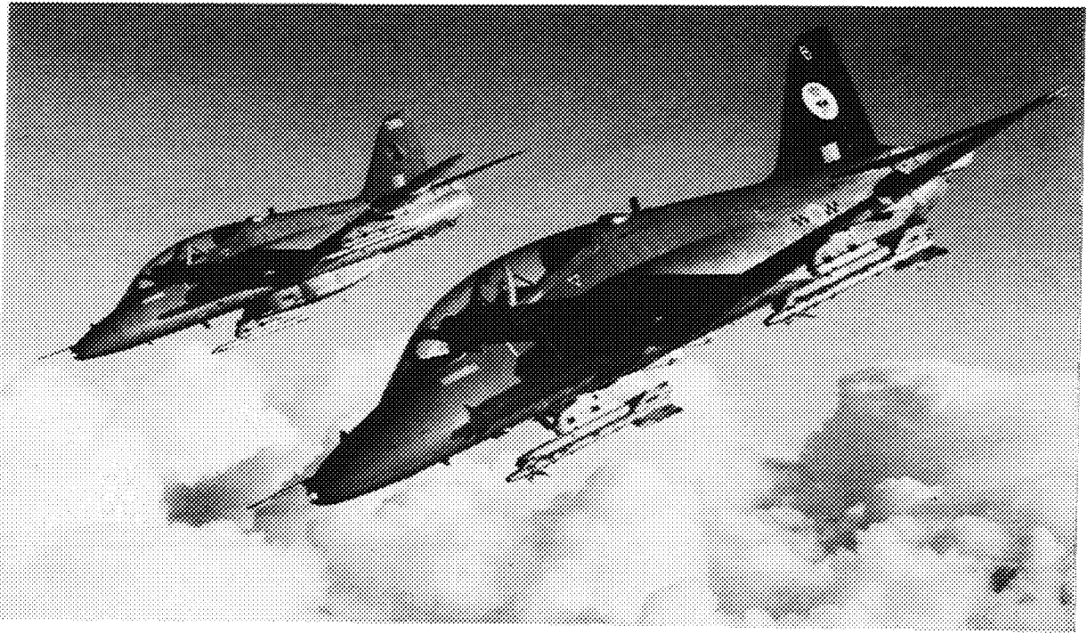
Figure 4. The loading spectrum experienced by the British Aerospace Hawk in the Tactical Weapons role is markedly more severe than that applied in the fatigue test and so a lower scatter factor is needed.
