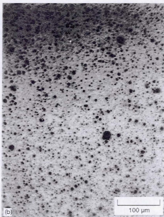
Figure 6.—Optical micrograph of thermal-energy atomic-oxygen exposed DC93-500 silicone samples whose surfaces are (a) smooth and (b) rough before the atomic oxygen exposure.
