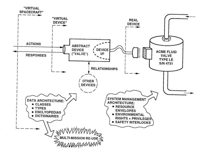
Figure 3. Device Model of Space Mission Control
