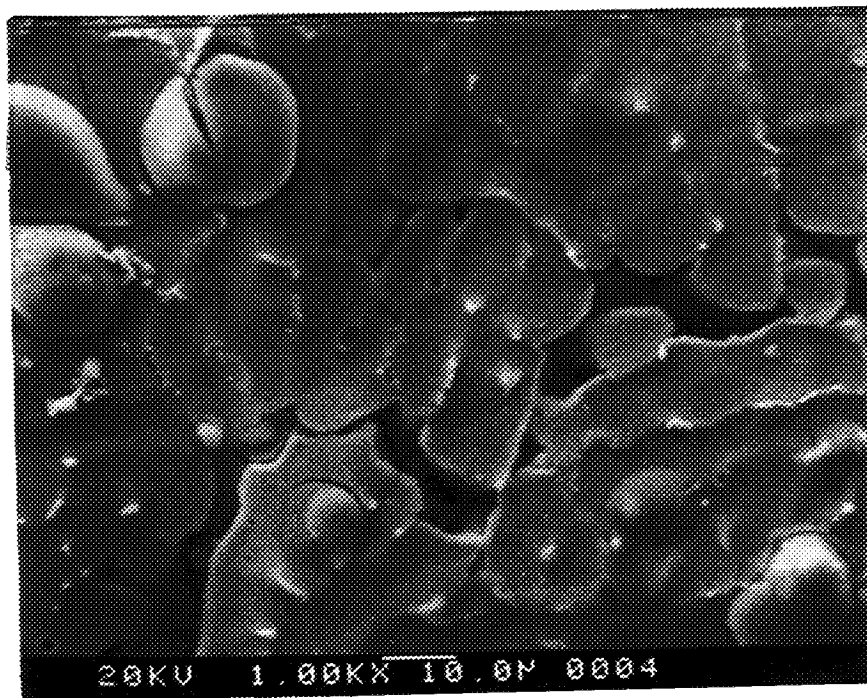
Figure 56 SEM Image of Al-Li cracking (without trailer).
