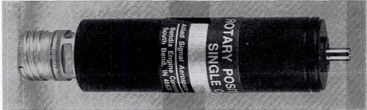
Figure 2.4-11. LEF Position Sensor (WDM Digital Code Plate, AlliedSignal)
