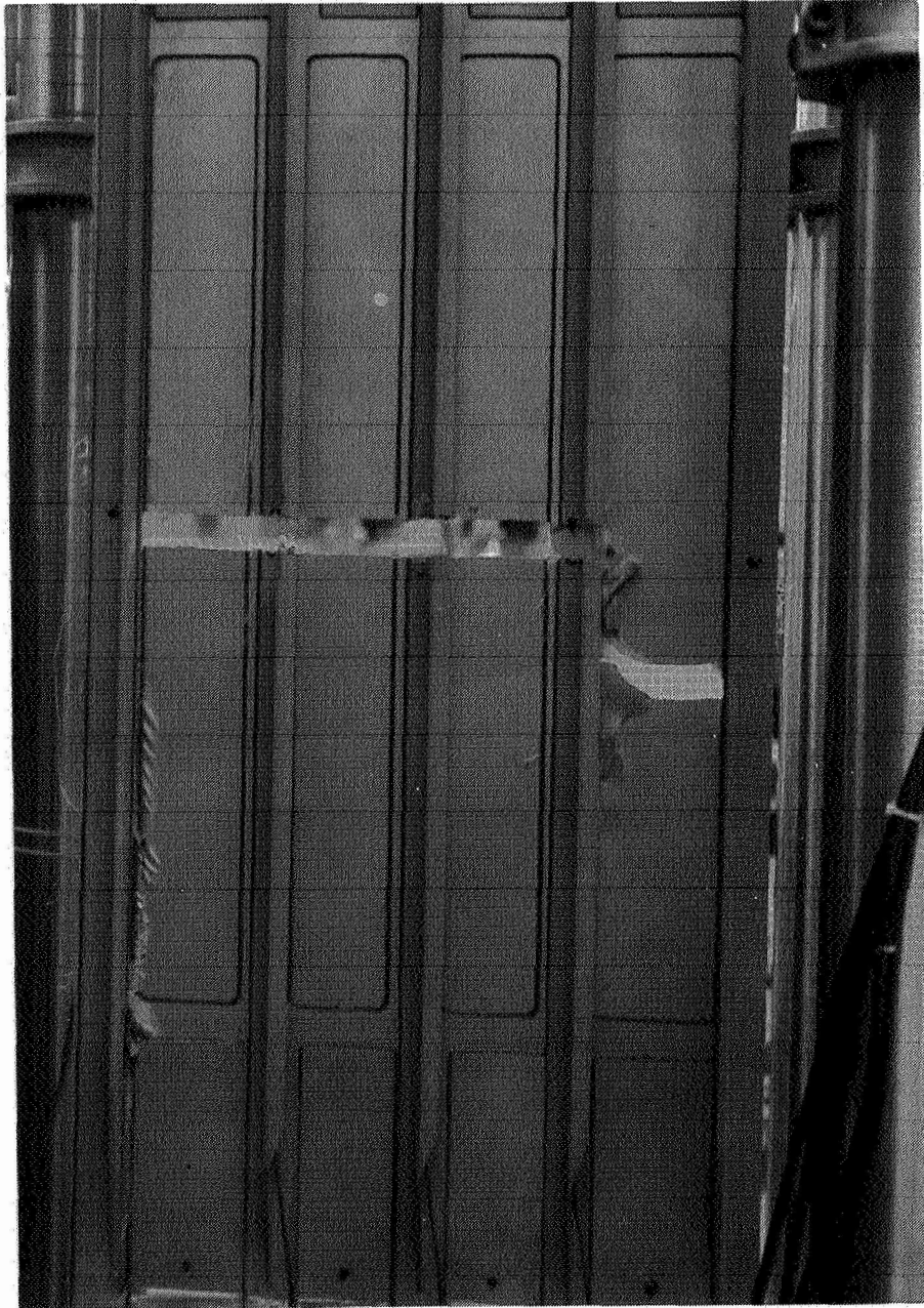
Figure 9: Stringer Side of Failed ARALL-3 Stiffened Panel.
