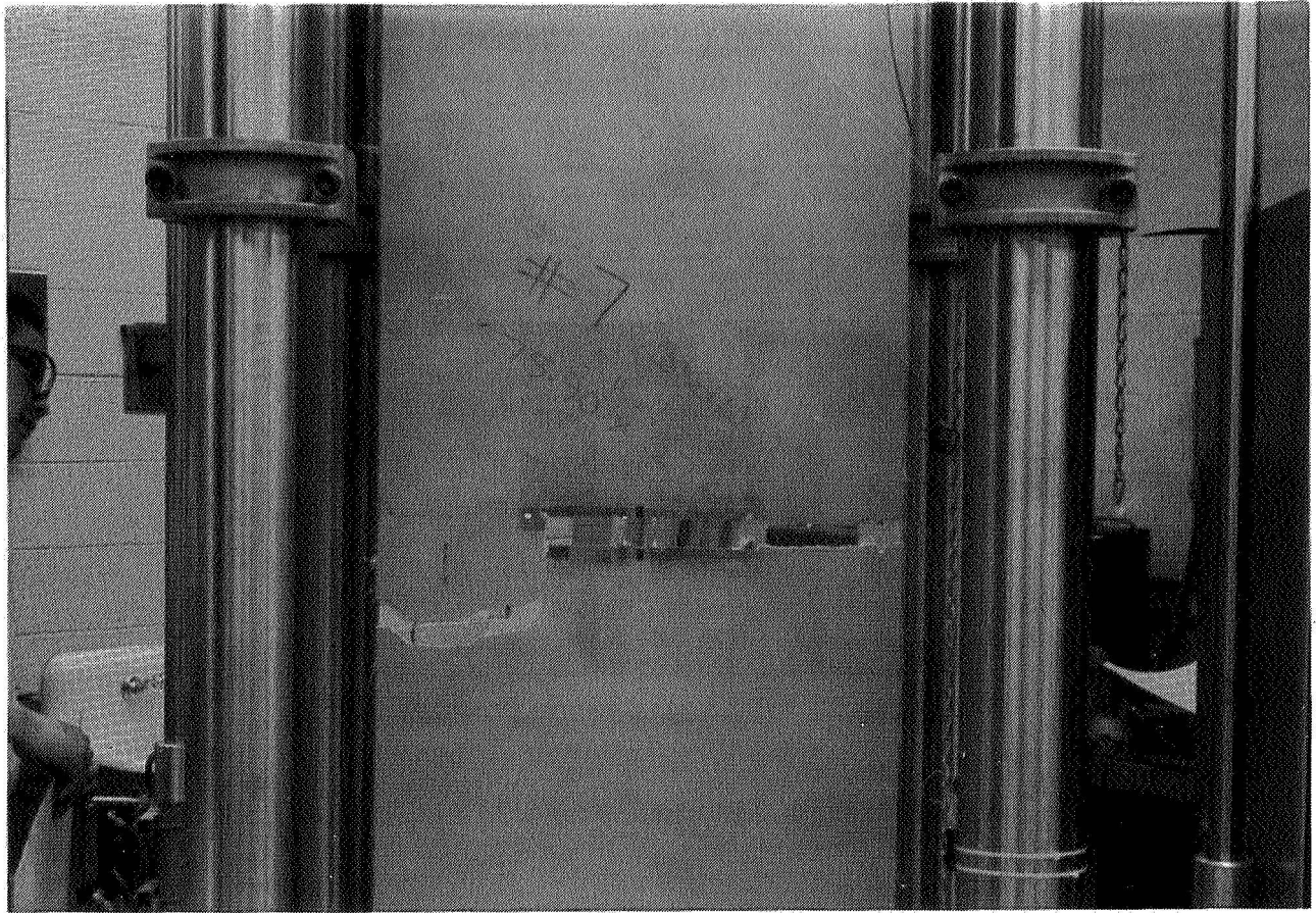
Figure 8: Skin Side of Failed ARALL-3 Stiffened Panel.
