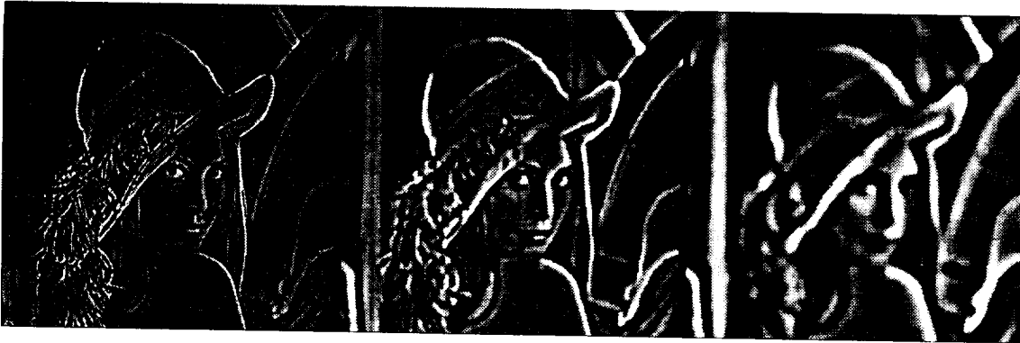
Fig. 2. Multiscale sequence of edge maps. Presented from left to right are the Laplacian pyramid components L_0 , L_1 , and L_2 , respectively. The pyramid components have been appropriately expanded to match in size.
