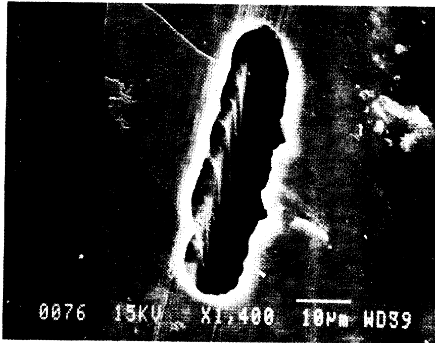
Figure 4. Undercut cavity associated with a wide defect in the aluminized Kapton after removal of the aluminized coating.
