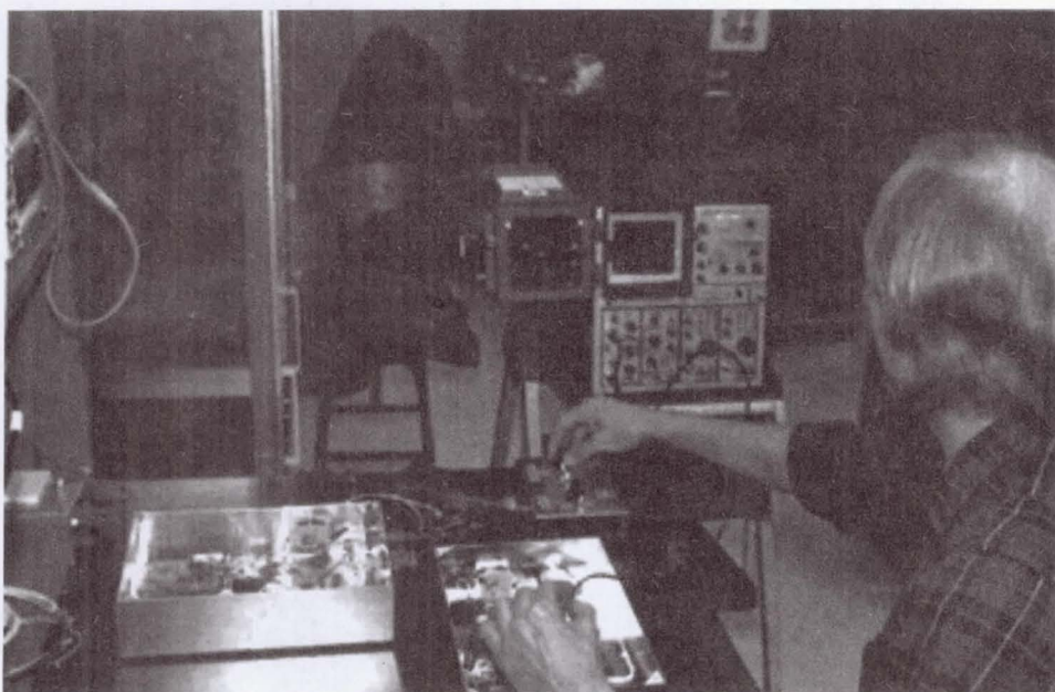
Breadboard supply for xenon ion thrusters.
