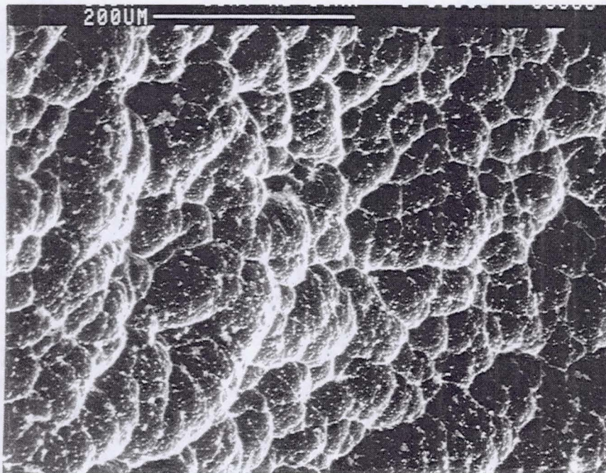
4b. After exposure to an effective atomic oxygen fluence of 2.9 \times 10^{21} atoms/cm 2 .
