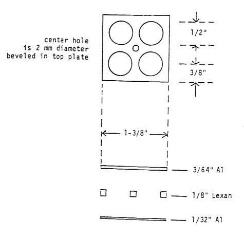
Fig. 6. Sketch of the <sup>232</sup>Th fission foil detector holders for K-7-41D. Two units, Fl and F2, were placed outside the spacecraft.
