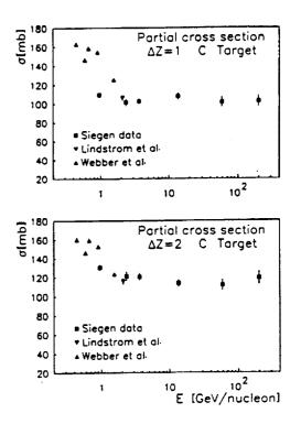
FIG. 8. Energy dependence of partial cross sections  $\Delta Z = 1$ (top) and  $\Delta Z = 2$  (bottom) for reaction of <sup>16</sup>O with carbon. Data from Webber, Kish, and Schrier [42,43] (triangles) and Lindstrom *et al.* [23] (inverted triangles) are also included.
