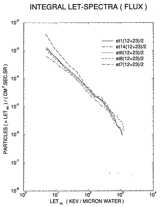
Fig. 2. Integral LET flux spectra from the EURECA Trackoscope. Spectra et1 and et14 are from opposing face PNTD stacks, as are et6 and et8. Spectra et1, -6, -7, -8 and -14 stacks are orthogonal in spatial orientation and show the effects of directionality of radiation in the EURECA satellite.
