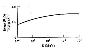
FIG. 1. Ratio of range in water to range in aluminum for proton beams.
