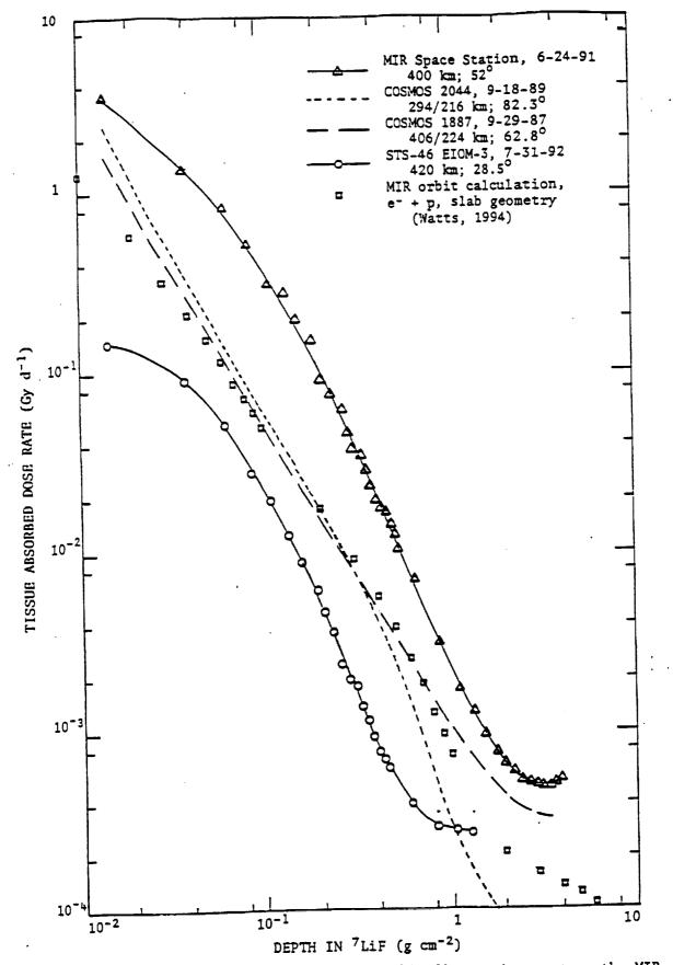
Fig. 5. TLD depth-dose rates measured in low shielding environment on the MIR space station (measured and calculated), Cosmos biosatellites Nos.1887 and 2044, and STS-46.
