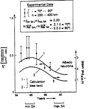
FIG. 2. The correlation of fast-neutron fluxes with solar activity (SA) phase in near-Earth orbits. Curve 1: calculated dependence of albedo neutron flux on SA cycle (Lingenfeiter, 1963). Curve 2: calculated relative time dependence of GCR particle flux (this paper).
