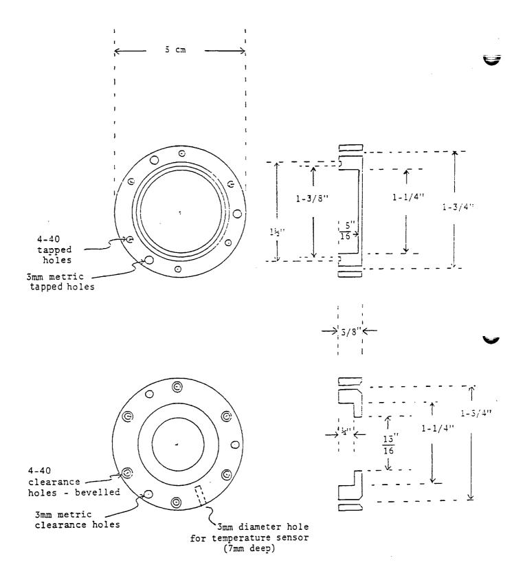
Fig. 3. Sketch of an aluminum container with O-ring seal for the plastic and emulsion stacks in K-7-41B. There were two flight units, Fl and F2 (outside the spacecraft). A double window of aluminized Kapton polyimide (total thickness: 15 µm) separated the stacks from space.
