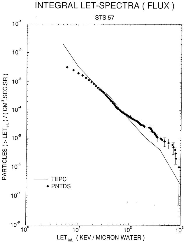
Fig. 8. Comparison of integral LET spectra measured by PNTDs and the TEPC microdosimeter on STS-57
