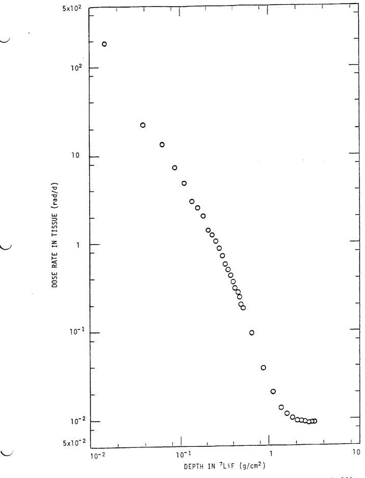
Fig. 11. Average dose rates in Plate No. B9-1 (TLD stacks Nos. 4, 8, 12) -20-
