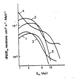
FIG. 1. Differential neutron energy spectra measured outside and inside the Soviet biosatellite Cosmos-2044. (1) Assembly No. 1 (outside); (2) assembly No. 2 (inside); (3) assembly No. 3 (outside); (4) assembly No. 4 (inside); (5) assembly No. 5 (outside).
