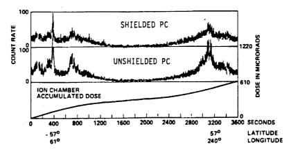
Fig. 16. One hour of ARD data in which the SAA and electron horns are not encountered. Large fluctuations in the PC count rates are likely due to electron precipitation.
