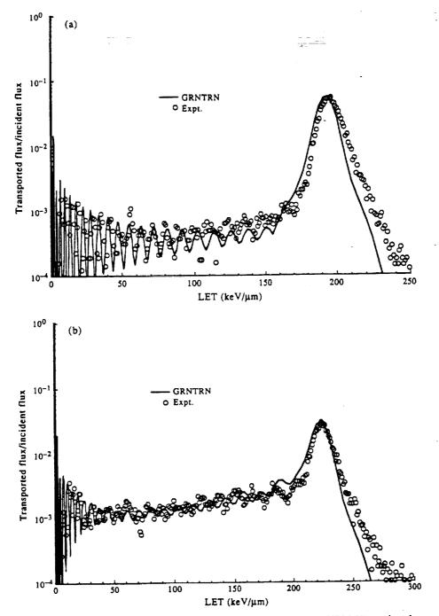
FIG. 6. Transport experiments for a lead-shield multilayer combination for 557 MeV/amu iron beams. (a) 2.24 g/cm<sup>2</sup> Pb + 2 g/cm<sup>2</sup> Al; (b) 2.24 g/cm<sup>2</sup> Pb + 4.6 g/cm<sup>2</sup> (CH<sub>2</sub>)<sub>x</sub>.
