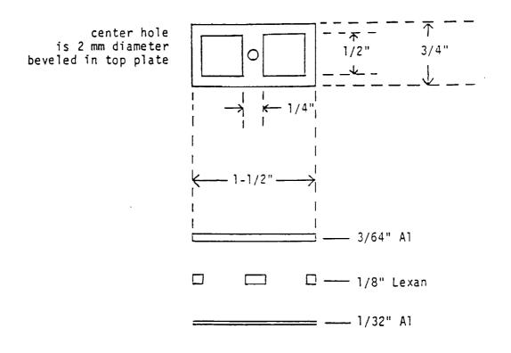
Fig. 7. Sketch of the <sup>6</sup>LiF/CR-39 neutron detector holders for K-7-41E. Each unit contained one unshielded detector and one shielded by 25 µm-thick Gd foil. Two units (F1 and F2) were placed outside the spacecraft.
