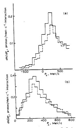
Fig. 3. The longitudinal (lab) (a) and transverse (b) momentum distributions of 30-400 MeV protons in the Fe+AgBr interactions. The dashed and solid-line histograms are the experimental and DCM calculation results, respectively.
