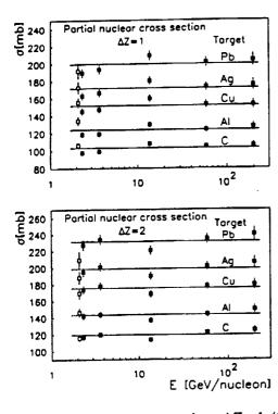
FIG. 3. Partial nuclear cross sections  $\Delta Z = 1$  (top) and  $\Delta Z = 2$  (bottom) for the reaction of <sup>16</sup>O with targets C, Al, Cu, Ag, and Pb determined from our experiments (solid squares) based on factorization rules. The data include cross sections from [41] at 2.1 GeV/nucleon (open squares). The horizontal line represents the average value of our cross-section data for all energies.
