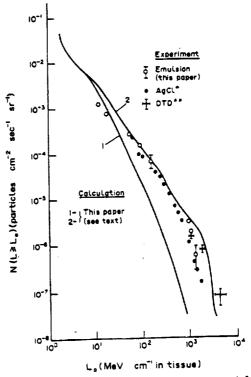
FIG. 5. Comparison of calculated and experimental LET distributions in investigations on board Cosmos-2044 (behind shielding of  $\delta > 10 \text{ g cm}^{-2}$ )—internal assemblies. [\*(AgCl): Baican et al., 1990; \*\*(DTD): Beaujean et al., 1990.]
