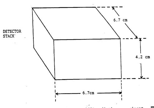
Fig.1 Detector components for EURECA radiation experiment. The Trackoscope base is a truncated cube with 7 pairs of parallel faces. PNTD sub-stacks (2.86 cm diam. x 0.25 cm thick) were placed on each of the 14 faces. The detector stack contained 6 additional TLD layers at various depths.
