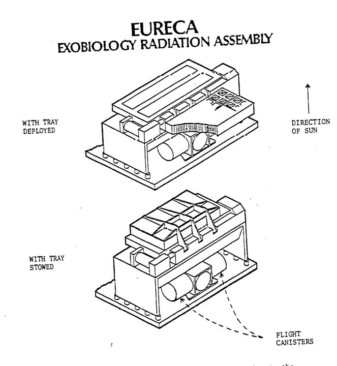
Fig. 3. The positions of flight canisters relative to the exobiology radiation assembly on the EURECA satellite
