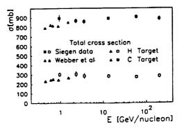
FIG. 6. Total charge-changing cross sections for <sup>16</sup>O for H and C targets. The squares (open for the H target, solid for the C target) represent our data, while the triangles give the data measured by Webber, Kish, and Schrier [42,43] (open triangle for the H target, solid triangle for the C target).
