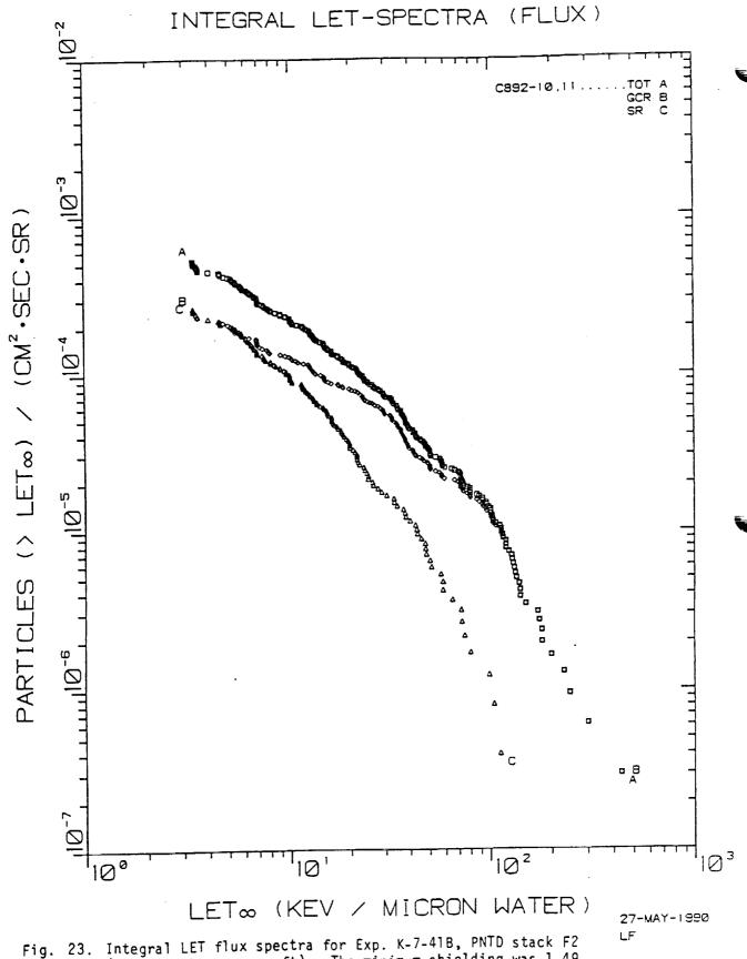
Fig. 23. Integral LET flux spectra for Exp. K-7-41B, PNTD stack F2 (outside the spacecraft). The minimum shielding was 1.49 g/cm<sup>2</sup> plastic, stainless steel and nuclear emulsion.
