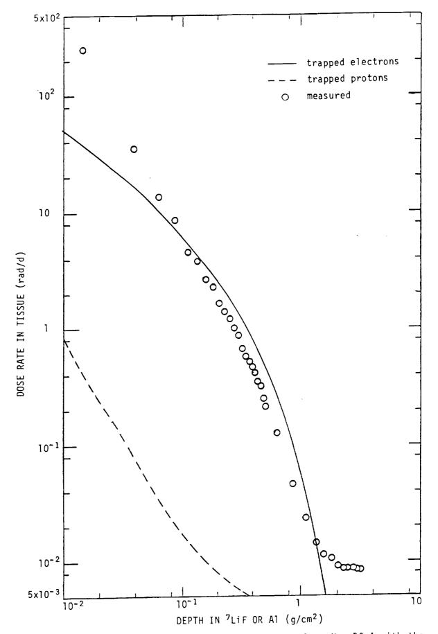
Fig. 25. Comparison of the average TLD dose rates in Plate No. B9-4 with the calculated depth dose rates of trapped electrons and protons for tissue behind aluminum plane shields /Watts, 1990/. The calculations were for the Cosmos 2044 orbit at solar maximum.
