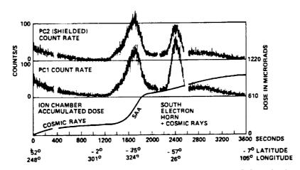
Fig. 15. Count rate of two proportional counters and ion chamber accumulation at high northern latitudes, the geomagnetic equator, the SAA, and the electron horn.
