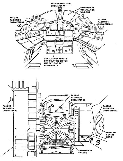
Fig. 7. Passive Radiation Detector locations on Space Shuttle. Top: aft flight deck Bottom: aft mid-deck /Atwell et al., 1987a/ nation flights was plotted as a function of orbital altitude and compared with calculations for solar minimum and solar maximum (see Fig. 10) /Atwell et al., 1987a/.
