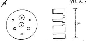
FIG. 1. Drawing, half actual size, of TLD stack container (Al) for Cosmos 1887 experiment. The U.S. detectors of  $0.32 \text{ cm} \times 0.32 \text{ cm}$  were in hole (a), U.S. detectors of  $0.64 \text{ cm} \times 0.64 \text{ cm}$  were in hole (b) and Soviet detectors of 0.8 cm diameter were in hole (c).
