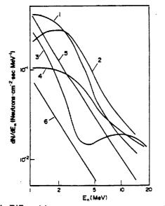
FIG. 1. Differential neutron energy spectra measured in spacecraft in low Earth orbit. Curves 1 and 2 are the Cosmos 1514 data obtained outside (1) and inside (2) the satellite. Curves 3 and 4 are the Cosmos 1887 data obtained outside (3) and inside (4) the satellite. Curves 5 and 6 are the albedo neutron spectra calculated in Lingenfelter (1963) at angle  $i = 90^{\circ}$  (5) and at  $i = 40^{\circ}$  (6) during solar minimum.
