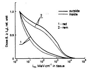
FIG. 3. The dose-LET distributions obtained on Cosmos-2044. The outside curves are for 1 g cm<sup>-2</sup> shielding; inside curves are for 20 g cm<sup>-2</sup>.
