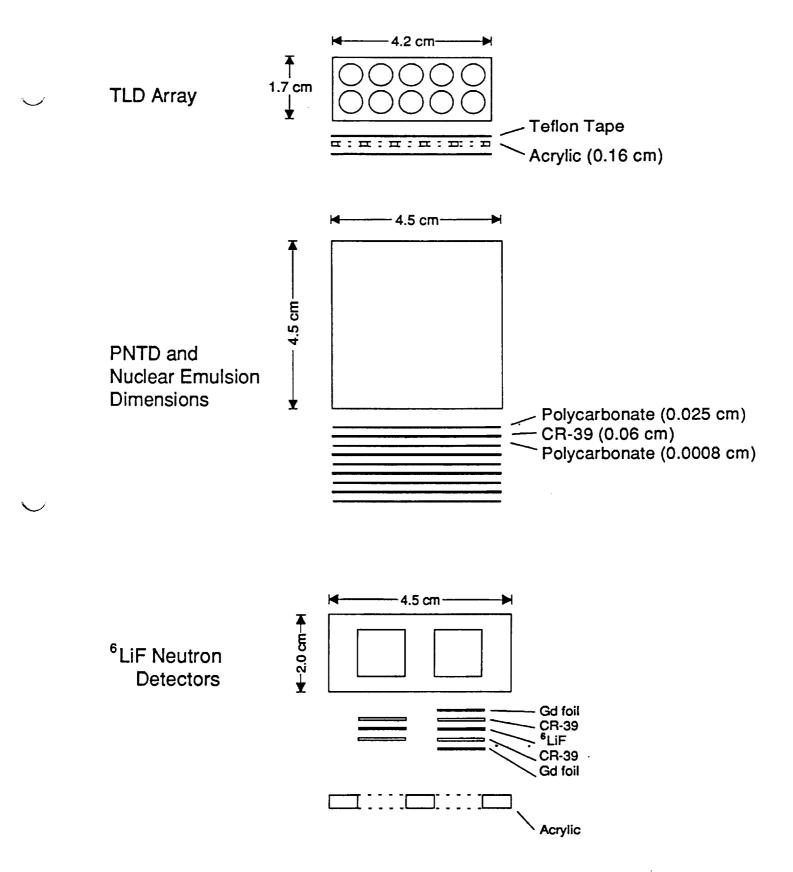
Figure 3: Dimensions of the TLD Array, PNTD center stack and TRND.
