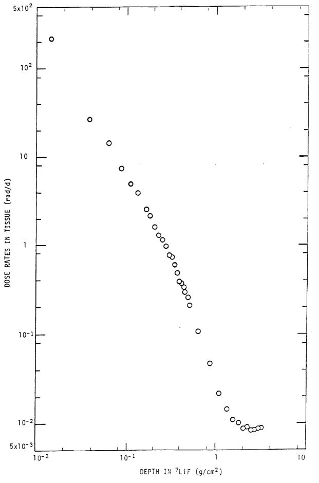
Fig. 12. Average dose rates in Plate No. B9-2 (TLD stacks Nos. 2, 6, 10) -21-
