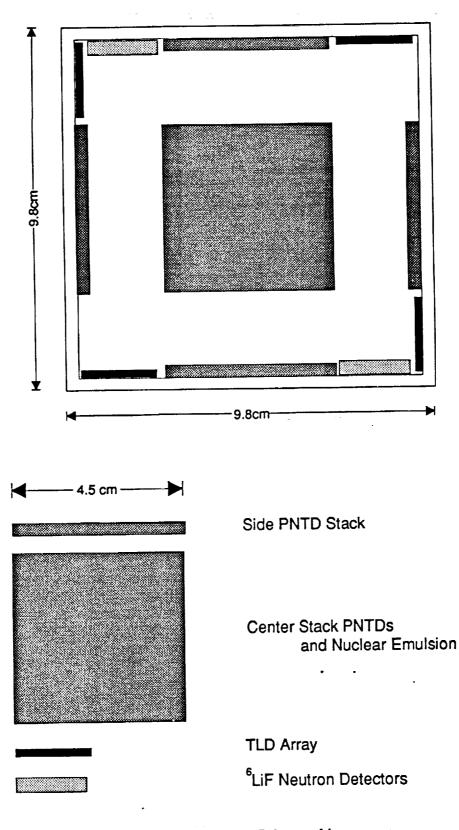
Figure 2: Top view of the APD box and its contents.
