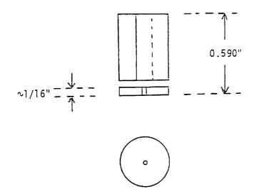
Fig. 1. Sketch of a TLD stack holder for K-7-41A, made of acrylate. Three stacks were placed in each of four plates (Plate No. B9-1, -2, -3, -4) for a total of twelve flight stacks (outside the spacecraft). A double window of aluminized Kapton polyimide (total thickness: 15 μm) separated the stacks from space.
