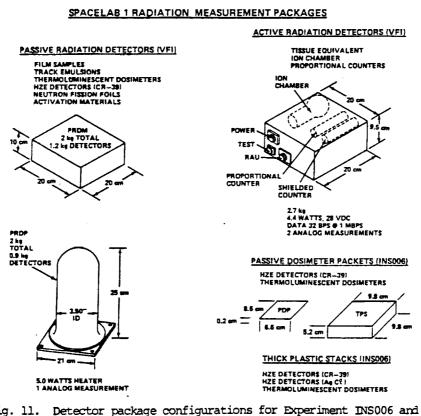
Fig. 11. Detector package configurations for Experiment INS006 and Verification Flight Instrumentation (VFI) on Spacelab-1 /Parnell et al., 1986/.
