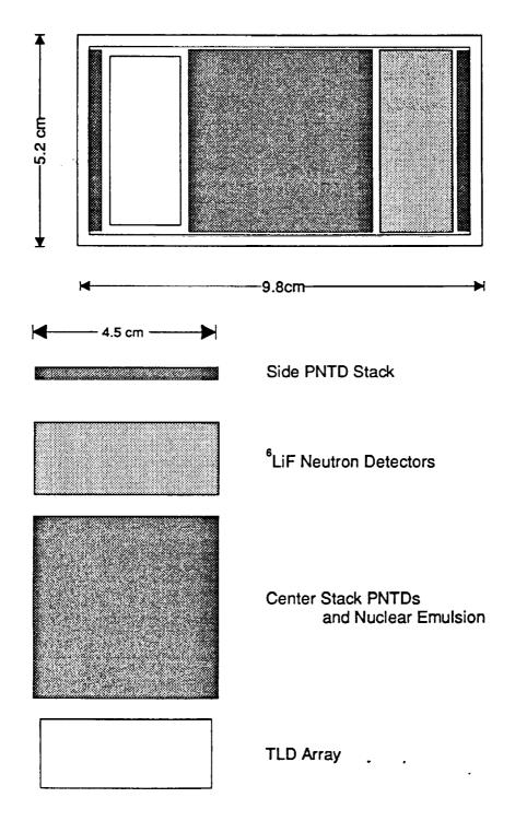
Figure 1: Side view of the APD box and its contents.
