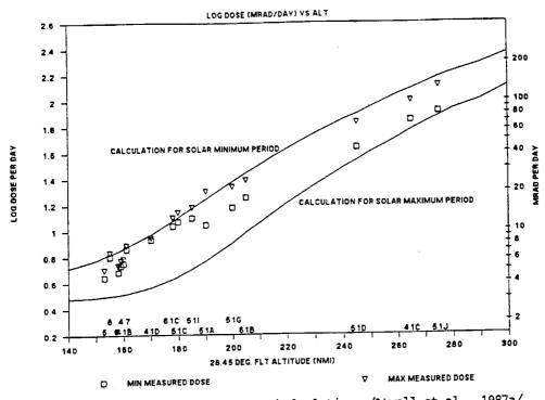
Fig. 10. STS PRD dose measurements/calculations /Atwell et al., 1987a/.
