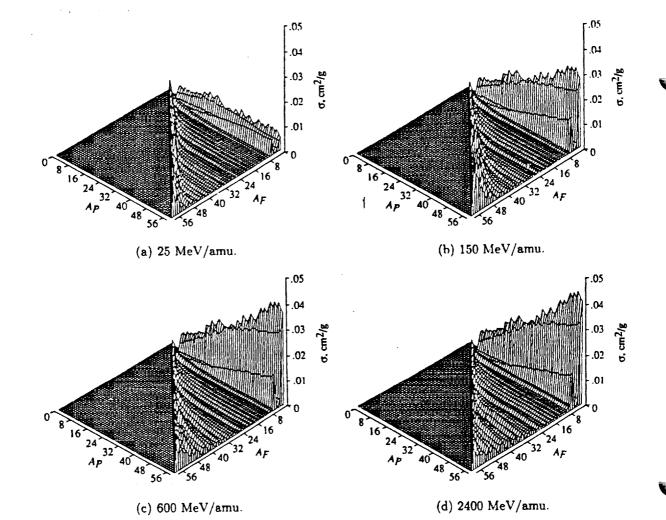
FIG. 4. The fragment production cross section in H<sub>2</sub>O targets including coulomb corrections.
