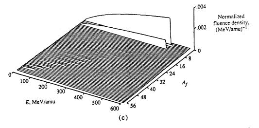
Fig. 2. Differential fluence for 525 MeV/amu <sup>56</sup>Fe beam with a 2.5 MeV/amu standard deviation after passing through a 2.24 g/cm<sup>2</sup> lead scattering foil and a water target. (a) 0 cm  $H_2O$ ; (b) 5 cm  $H_2O$ ; (c) 10 cm  $H_2O$ .
