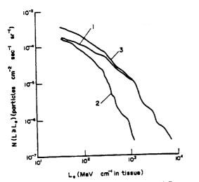
FIG. 2. Integral LET spectrum measured on board Cosmos-2044 with CR-39 track detectors behind  $\delta = 1.95$  g cm<sup>-2</sup>.
