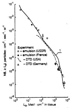
FIG. 1. Comparison between the calculated (curve 1—for  $l \ g \ cm^{-2}$ ) and experimental integral LET distributions of CR particles obtained on Cosmos-2044 (stacks outside the satellite); DTD denotes plastic dielectric track detectors.
