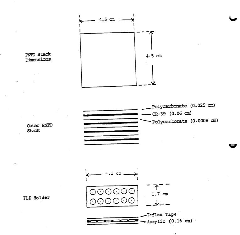
Fig. 6. Dimensions and components of the outer PNTD stacks and the TLD holder - PNTD #5717
