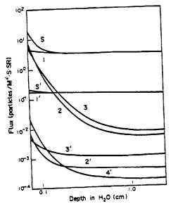
FIG. 2. The calculated flux vs detector depth. Curves 1-4 are particle fluxes calculated by formulas (8)-(11), respectively. S is the total particle flux with  $L > L_o$  at depth x. The curves numbered without a prime are for L > 40 MeV cm g<sup>-1</sup>; those with a prime are for L > 1000 MeV cm g<sup>-1</sup>. Curve 4' is not present for the values of LET and plastic thickness used.
