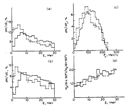
Fig. 4. The characteristics of  $E_p \le 30$  MeV protons in the Fe+AgBr interactions: the energy spectra at forward (a) and backward (b) hemispheres; the transverse-momentum distribution (c), and the "forward-to-backward" ratio energy dependence (d), the dashed and solid-line histograms are the experimental and DCM calculation results, respectively.
