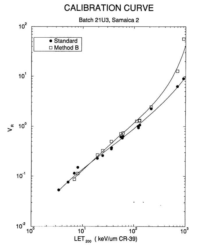
Fig. 3. A comparison of PNTD calibration curves for the Standard and Method B processing conditions. Method B was developed to enhance PNTD sensitivity for short range (8-80 µm) particle tracks.
