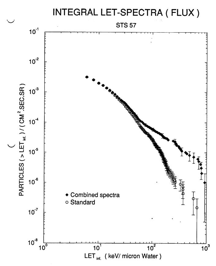
Fig. 1. Comparison of the standard and combined integral LET spectra on the STS-57 APD.
